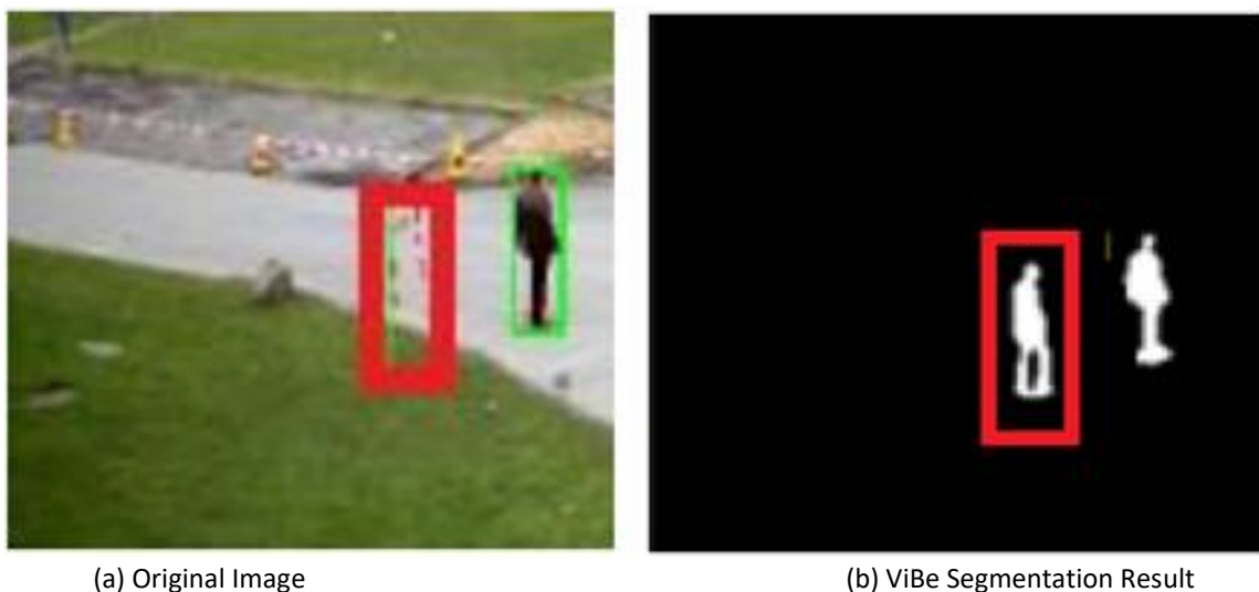
Figure 2.3. The appearance of a ghost in ViBe background subtraction result in [63]. only one person exists in the scene, but ViBe detected two moving objects, the ghost area manually marked with a red rectangle in both images.
