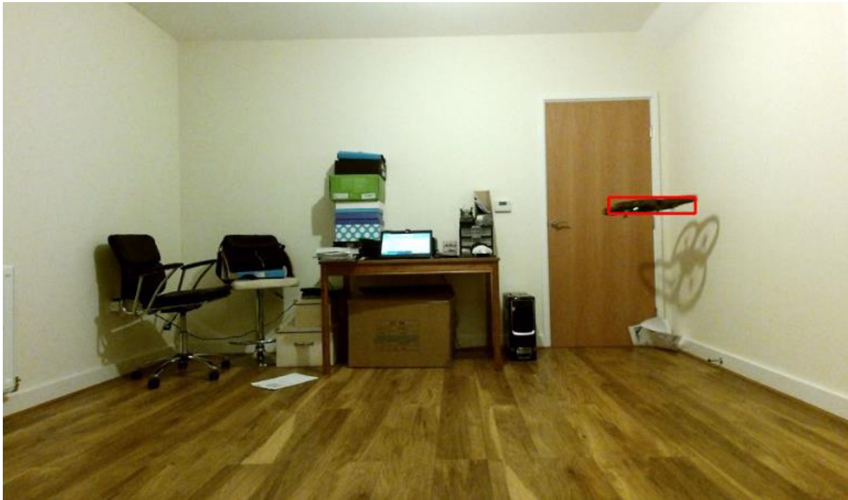
Figure 3.10. Detection accuracy in the appearance of a shadow. Red rectangle illustrates the detected foreground region.
