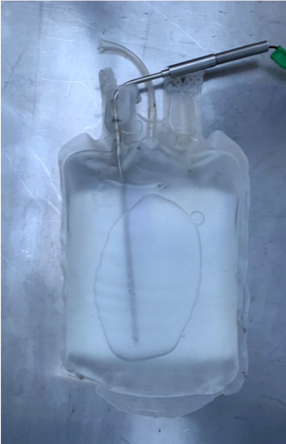
Figure 5-17: Installed thermocouple in plasma bag
