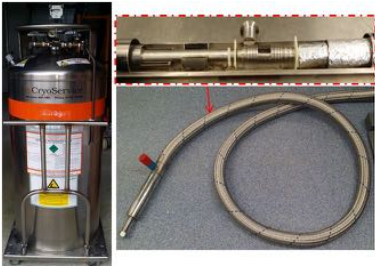
Figure 5-6: (a) Liquid nitrogen supply tank (b) Vacuum insulated hose (c) Interior of vacuum insulated hose
