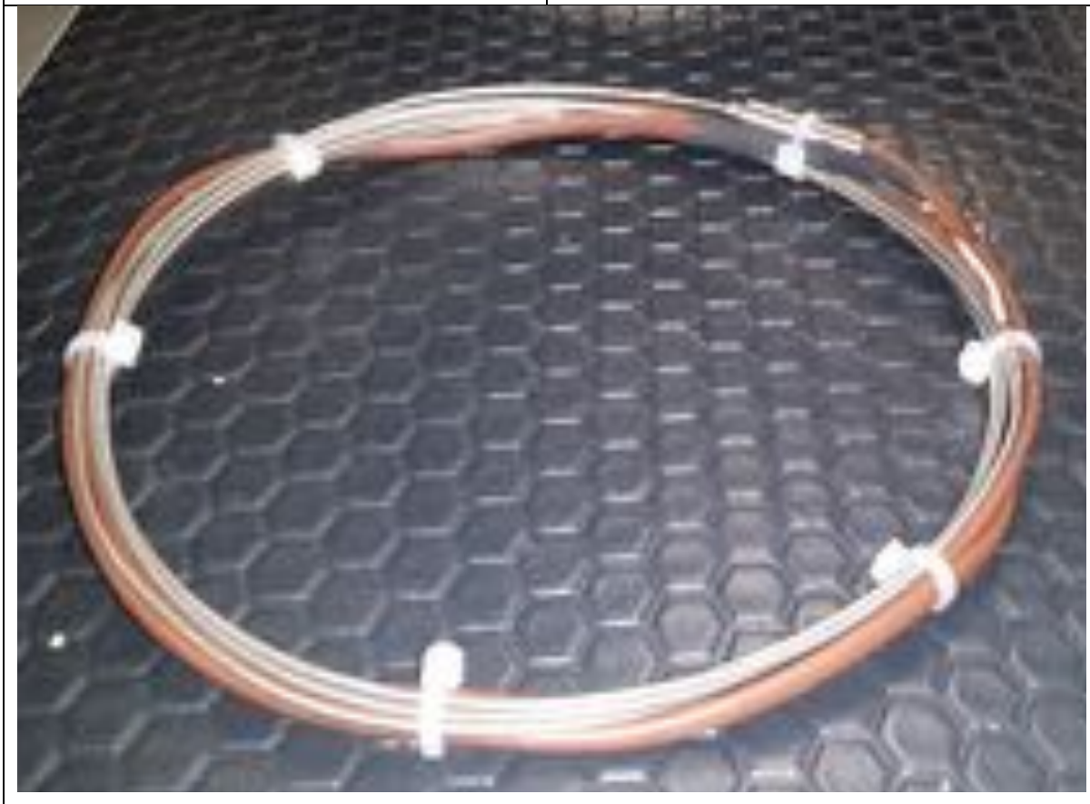
Figure 5-8: Thermocouple probe details
