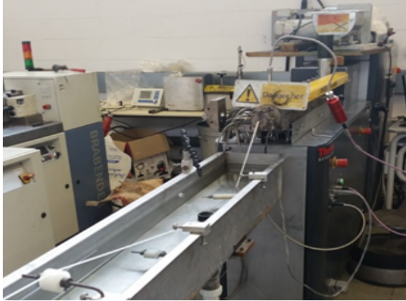
Figure 1. 25mm twin screw extruder used for polymer/starch composite processing.
