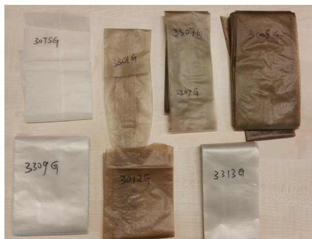
Figure 7. Blown film sample from blends of polymer with reclaimed starches.
