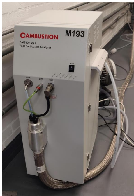
Figure 3-15 Cambustion DMS500 MkII fast particle analyser
