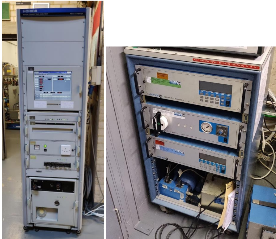
Figure 3-13 Horiba MEXA7170D-EGR and Signal group gas analyser unit
