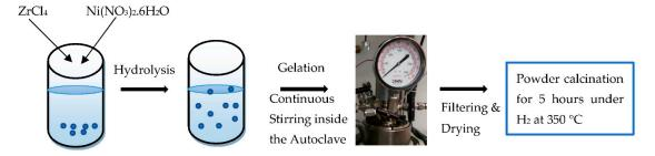
Figure 11. The steps of synthesis of the catalyst preparation.
