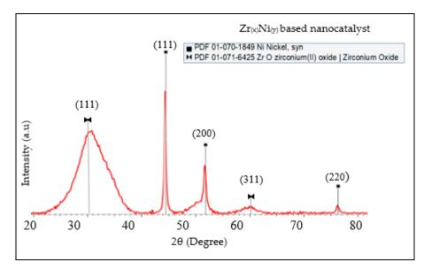
**Figure 1.** The XRD patterns of  $Zr_{(x)}Ni_{(y)}$  based nanocatalyst.
