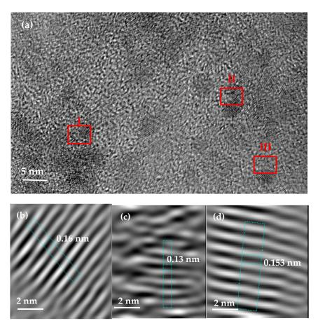
**Figure 2.** Field emission high resolution transmission electron microscopy (FE-HRTEM). (a)  $Zr_{(x)}Ni_{(y)}$  nanocatalyst, (b) the lattice image of zone I; (c) the lattice image of zone II; (d) the lattice image of zone III.
