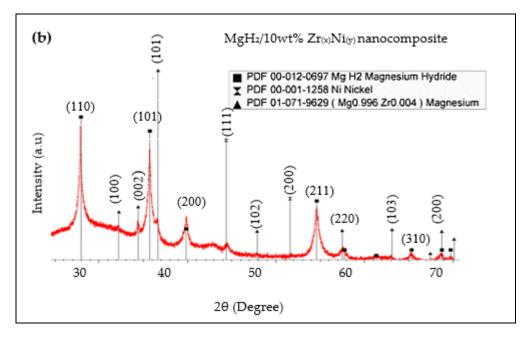
**Figure 5.** The XRD patterns of (**a**) 10 wt.%  $Zr_{(x)}Ni_{(y)}$  nanocomposite in red and the un-milled MgH<sub>2</sub> used as reference in black and (**b**) MgH<sub>2</sub>/10 wt.%  $Zr_{(x)}Ni_{(y)}$  nanocomposite to identify the crystal phase of each element.
