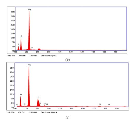
**Figure 8.** The energy dispersive X-ray spectrocopy (EDX) of (**a**)  $Zr_{(x)}Ni_{(y)}$  nanocatalyst; (**b**) milled-MgH<sub>2</sub> as reference; (**c**) MgH<sub>2</sub>/10 wt.%  $Zr_{(x)}Ni_{(y)}$  nanocomposite.
