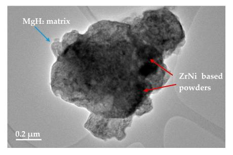
**Figure 10.** TEM of the bright field image of  $MgH_2$  powders milled with  $10 \text{ wt.} \% Zr_{(x)}Ni_{(y)}$ , demonstrating the agglomeration of catalyst on the surface of the  $MgH_2$  matrix after 5 h milling time.
