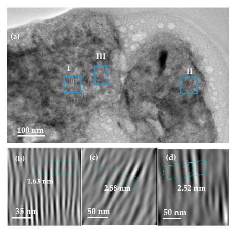
**Figure 9.** Field emission high resolution transmission electron microscopy (FE-HRTEM) of (a)  $MgH_2/10$  wt.%  $Zr_{(x)}Ni_{(y)}$  nanocomposite; (b) the lattice image of zone I; (c) the lattice image of zone II; (d) the lattice image of zone III.
