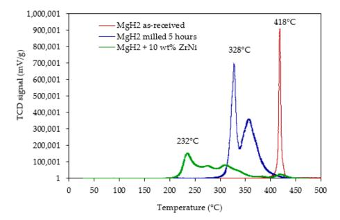
**Figure 3.** The evolution of the temperature-programmed desorption (TPD) profile of as-received MgH<sub>2</sub> after milling without/with 10 wt.%  $Zr_{(x)}Ni_{(y)}$ . Experimental conditions: from ambient temperature to 500 °C under an argon flow of 20 mL min<sup>-1</sup> and at a heating rate of 2 °C min<sup>-1</sup>.
