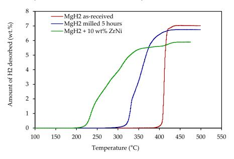
**Figure 4.** Thermally programmed H<sub>2</sub> desorption capacity curves of studied powders. Same experimental conditions as given in Figure 3.
