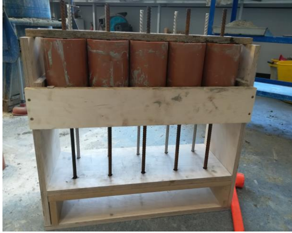
Fig. 6.5: Photo of the rig used for casting pull-out specimens.
