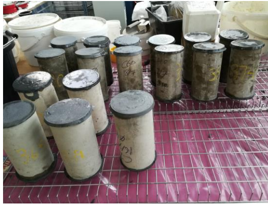
Fig. 6.3: Cylindrical concrete samples capped with sulphur.
