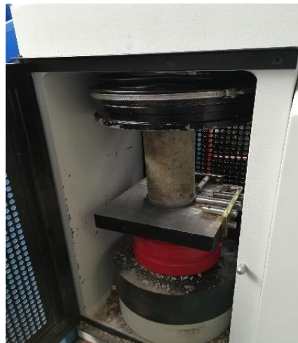
Fig. 6.2: Concrete compression testing machine.
