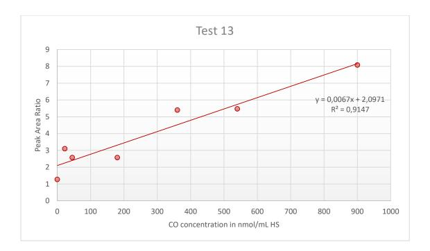
**Figure A3.13:** Peak Area Ratio of carbon monoxide (CO) from the blood sample over <sup>13</sup>CO from the internal standard (IS) plotted against the CO concentration in the calibration standards, with addition of linear trendline, linear regression equation and regression coefficient ( $R^2$ ) for Test 13.
