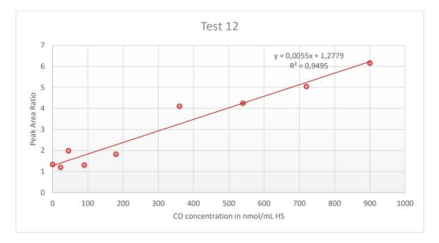
**Figure A3.12:** Peak Area Ratio of carbon monoxide (CO) from the blood sample over <sup>13</sup>CO from the internal standard (IS) plotted against the CO concentration in the calibration standards, with addition of linear trendline, linear regression equation and regression coefficient ( $R^2$ ) for Test 12.
