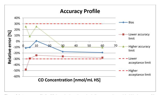
**Figure 3.4:** Accuracy profile for CO determination using a simple linear regression model within the range of 2-60 nmol/mL HS (0.8-24  $\mu$ mol/mL blood). The continuous line represents the trueness (bias), the dashed lines represent the acceptance limits set at  $\pm$  30% and the dotted lines are the relative lower and upper accuracy limits.
