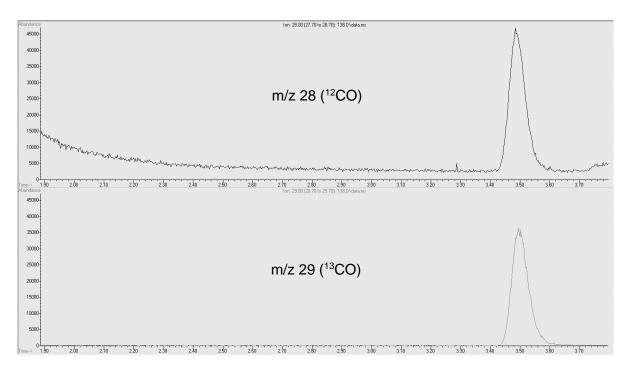
**Figure 3.1:** Extracted ion chromatograms for m/z ratios 28 (upper) and 29 (lower), corresponding to CO and 13CO respectively, for selectivity tests.
