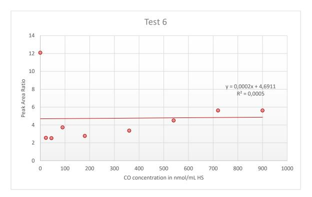
**Figure A3.6:** Peak Area Ratio of carbon monoxide (CO) from the blood sample over <sup>13</sup>CO from the internal standard (IS) plotted against the CO concentration in the calibration standards, with addition of linear trendline, linear regression equation and regression coefficient ( $R^2$ ) for Test 6.
