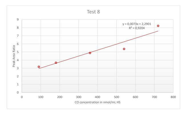
**Figure A3.8:** Peak Area Ratio of carbon monoxide (CO) from the blood sample over <sup>13</sup>CO from the internal standard (IS) plotted against the CO concentration in the calibration standards, with addition of linear trendline, linear regression equation and regression coefficient ( $R^2$ ) for Test 8.
