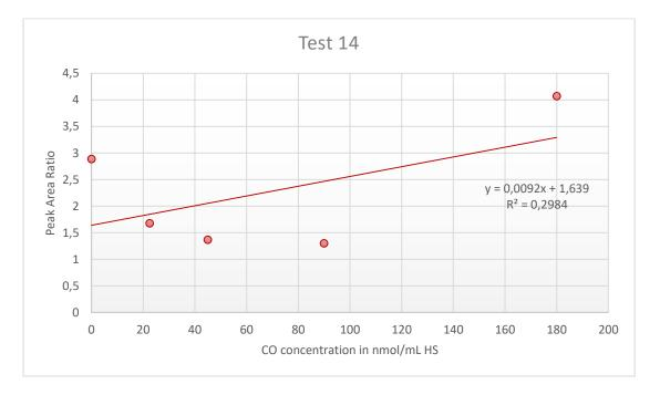
**Figure A3.14:** Peak Area Ratio of carbon monoxide (CO) from the blood sample over <sup>13</sup>CO from the internal standard (IS) plotted against the CO concentration in the calibration standards, with addition of linear trendline, linear regression equation and regression coefficient ( $R^2$ ) for Test 14.
