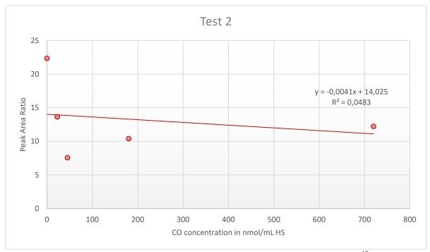
**Figure A3.2:** Peak Area Ratio of carbon monoxide (CO) from the blood sample over <sup>13</sup>CO from the internal standard (IS) plotted against the CO concentration in the calibration standards, with addition of linear trendline, linear regression equation and regression coefficient ( $R^2$ ) for Test 2.
