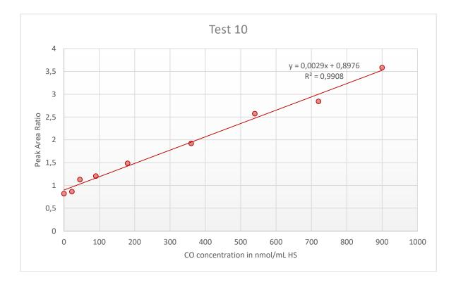
**Figure A3.10:** Peak Area Ratio of carbon monoxide (CO) from the blood sample over <sup>13</sup>CO from the internal standard (IS) plotted against the CO concentration in the calibration standards, with addition of linear trendline, linear regression equation and regression coefficient ( $R^2$ ) for Test 10.
