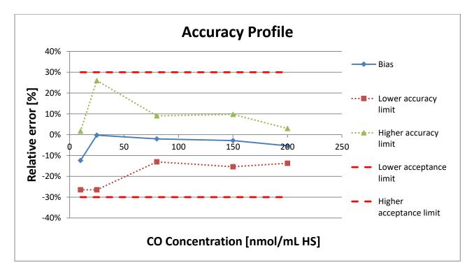
**Figure 3 2:** Accuracy profile for CO determination using a simple linear regression model within the range of 10-200 nmol/mL HS (2-40  $\mu$ mol/mL blood). The continuous line represents the trueness (bias), the dashed lines represent the acceptance limits set at  $\pm$  30% and the dotted lines are the relative lower and upper accuracy limits.
