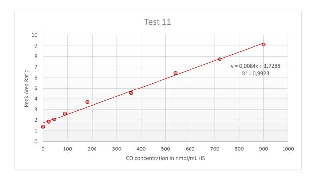
**Figure A3.11:** Peak Area Ratio of carbon monoxide (CO) from the blood sample over <sup>13</sup>CO from the internal standard (IS) plotted against the CO concentration in the calibration standards, with addition of linear trendline, linear regression equation and regression coefficient ( $R^2$ ) for Test 11.
