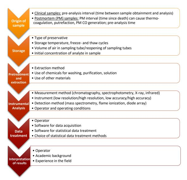
**Figure 2.1:** General steps for quantitative laboratory analysis and their respective potential sources of error for CO determinations.
