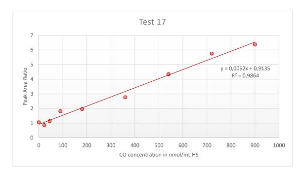
**Figure A3.17:** Peak Area Ratio of carbon monoxide (CO) from the blood sample over <sup>13</sup>CO from the internal standard (IS) plotted against the CO concentration in the calibration standards, with addition of linear trendline, linear regression equation and regression coefficient ( $R^2$ ) for Test 17.
