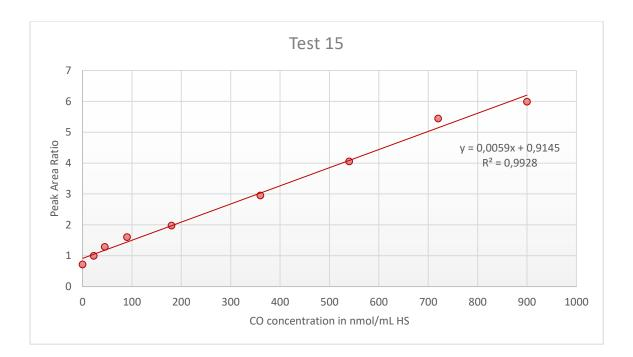
**Figure A3.15:** Peak Area Ratio of carbon monoxide (CO) from the blood sample over <sup>13</sup>CO from the internal standard (IS) plotted against the CO concentration in the calibration standards, with addition of linear trendline, linear regression equation and regression coefficient ( $R^2$ ) for Test 15.
