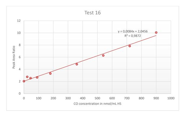
**Figure A3.16:** Peak Area Ratio of carbon monoxide (CO) from the blood sample over <sup>13</sup>CO from the internal standard (IS) plotted against the CO concentration in the calibration standards, with addition of linear trendline, linear regression equation and regression coefficient ( $R^2$ ) for Test 16.
