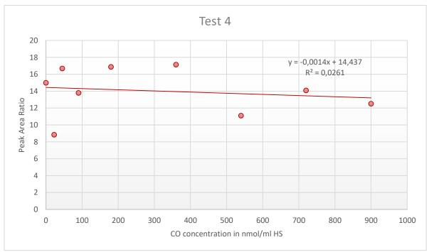
**Figure A3.4:** Peak Area Ratio of carbon monoxide (CO) from the blood sample over <sup>13</sup>CO from the internal standard (IS) plotted against the CO concentration in the calibration standards, with addition of linear trendline, linear regression equation and regression coefficient ( $R^2$ ) for Test 4.
