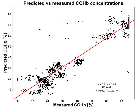
**Figure 4.4:** Correlation plot for measured COHb vs predicted COHb concentrations in %. Complete dataset was subdivided in training (2/3) and test (1/3) set, prediction model was generated based on training set and applied to test set and plotted to determine applicability and accuracy of prediction model.
