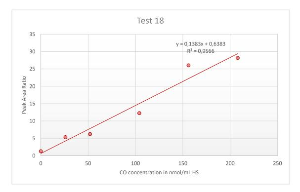
**Figure A3.18:** Peak Area Ratio of carbon monoxide (CO) from the blood sample over <sup>13</sup>CO from the internal standard (IS) plotted against the CO concentration in the calibration standards, with addition of linear trendline, linear regression equation and regression coefficient ( $R^2$ ) for Test 18.
