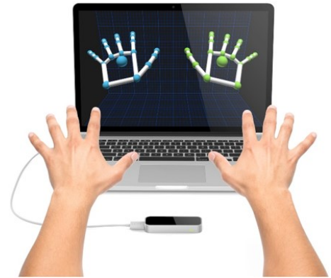
Figure 1.4: Leap Motion sensor capture hand motion by the skeleton[2]
