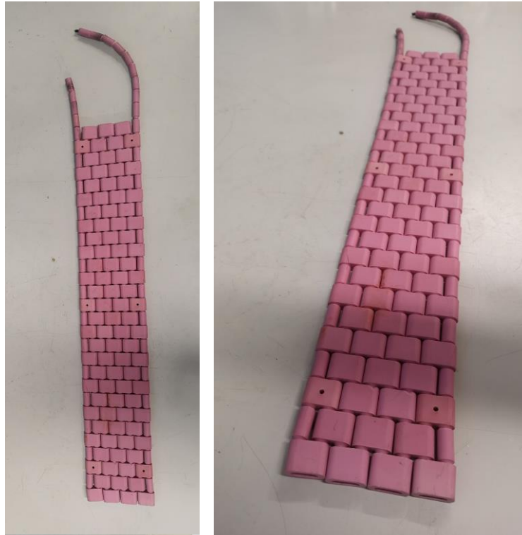
Figure 3-7 Picture of the electrical heaters used in the kiln
