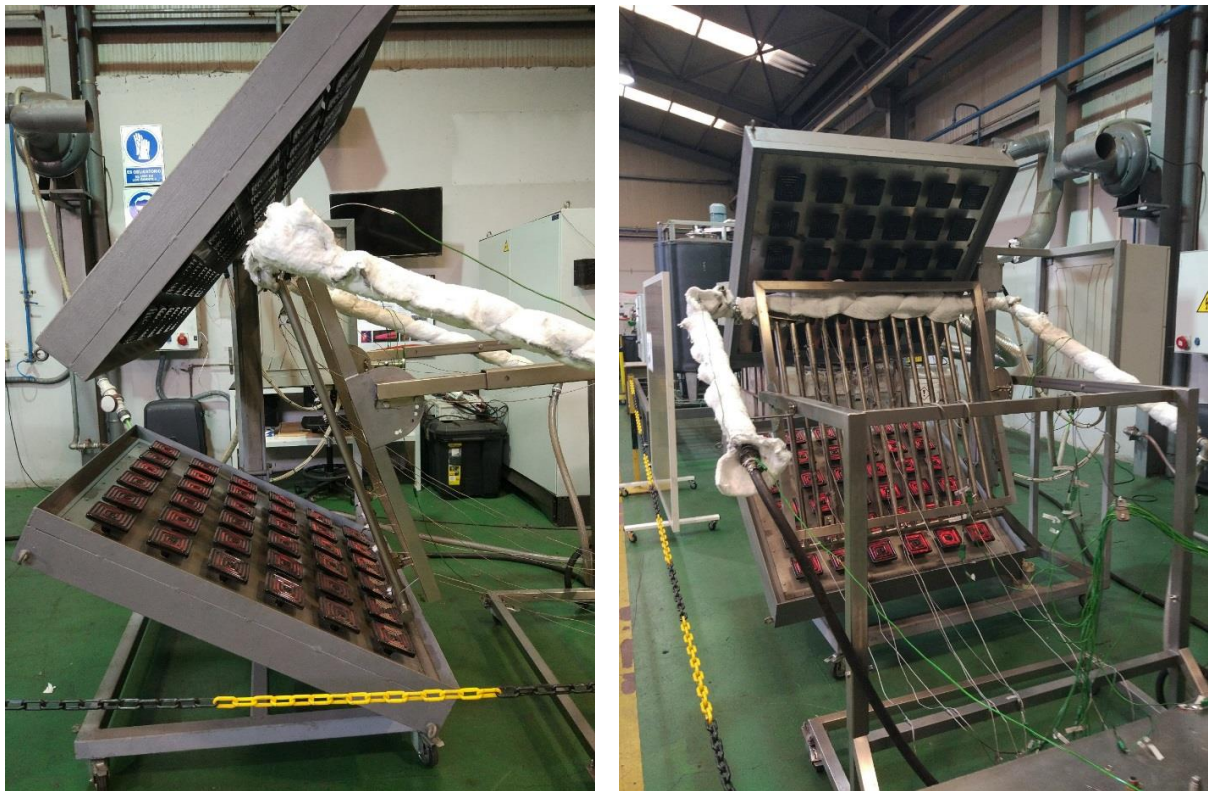
Figure 3-44 FHP laboratory testing without back panel and no paint
