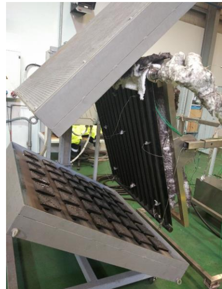
Figure 3-48 FHP laboratory testing with a back panel and black paint, water inlet temperature 70 °C
