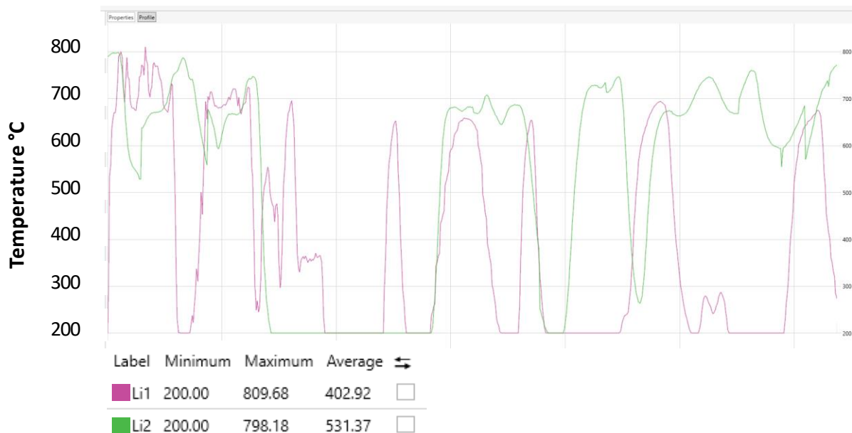
Figure A2-17 Temperature profile from line 1 and line 2 of the steel thermal image at position 3
