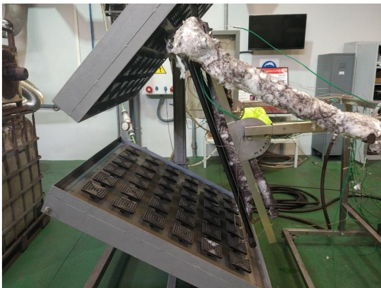
Figure 3-48 FHP laboratory testing with a back panel and black paint, water inlet temperature 70 °C
