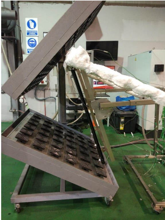
Figure 3-47 FHP laboratory testing with a back panel and black paint
