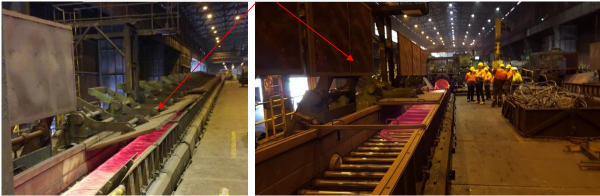
Figure 3-58 Moving covers for steel quality control
