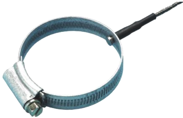
Figure 3-36 Thermocouple K-type used in FHP experiments
