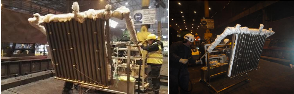
Figure 3-60 Flat Heat Pipe set-up at factory tests
