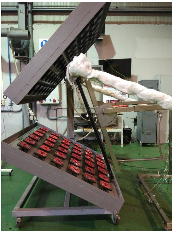
Figure 3-46 FHP laboratory testing without back panel and painted black
