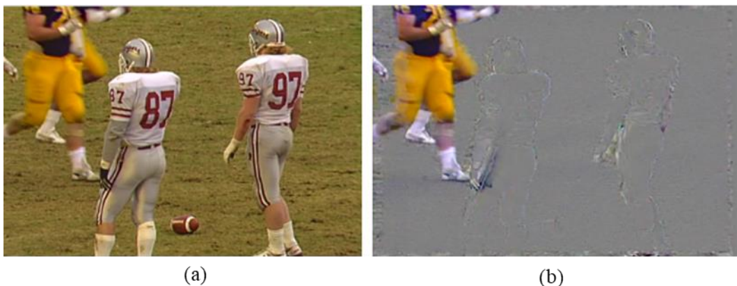
Figure 2.6 Error propagation effect caused by one-bit error (a) original frame, (b) Erroneous frame [34]
