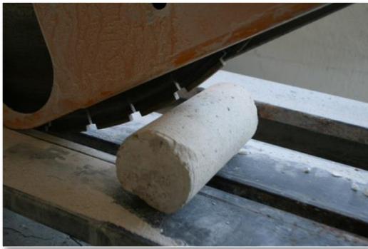
Figure 5 -2: Cutting samples with the use of a circular saw
