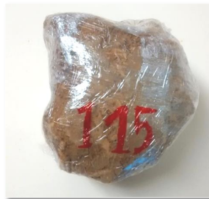
Figure 5 -6: Sample covered with nylon foil
