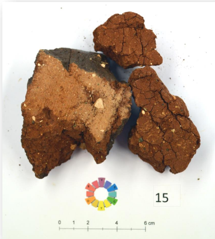
Sample 015 - Reddish brown sandy clay with gravel, Fluvial deposits
