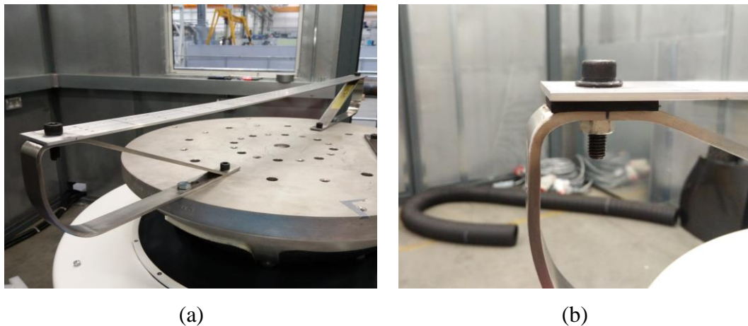
Figure 5-1 (a) A 6082-T6 aluminium plate fixed at both ends. (b) A 10mm diameter bolt is covered with rubber mount and sleeves to avoid noise generated at the supports.
