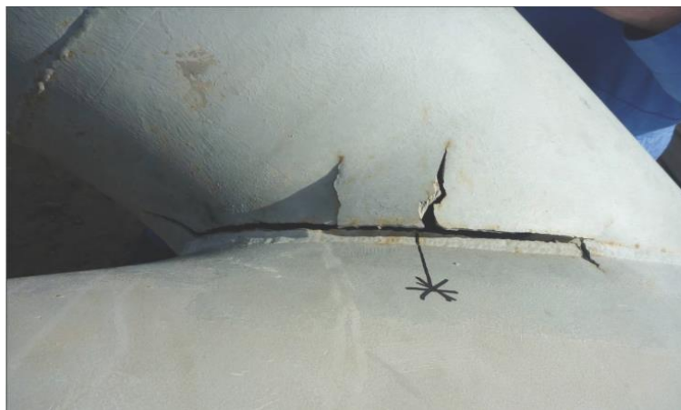
Figure 1-2 Fatigue crack due to acoustic induced vibration [8]
