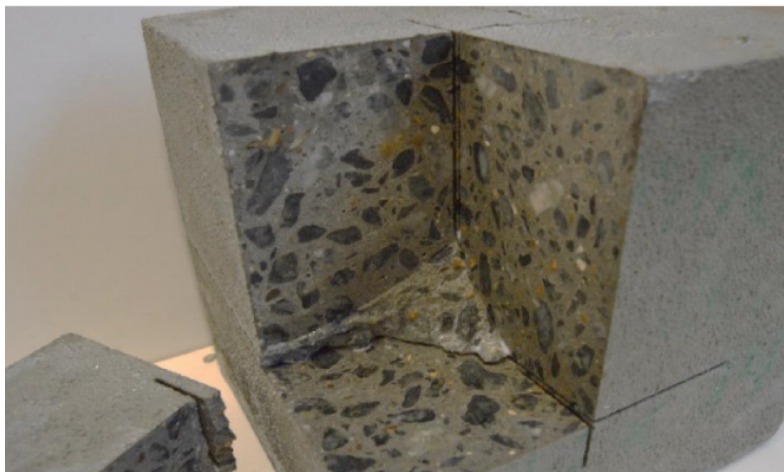
Figure 5-2 - Concrete with w/c ratio of 0.48 and treated with 8% crystalline material without any visible cracks or segregation
