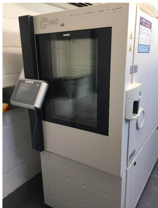
Figure 3-10 - Freeze-thaw chamber for testing concrete under the effect of water
