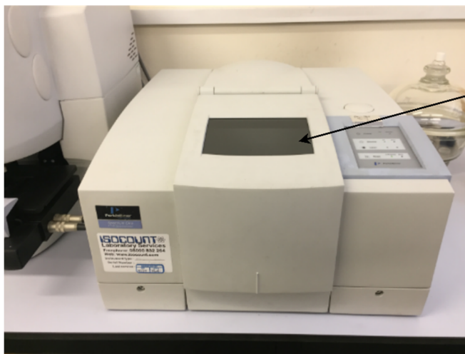
Figure 3-18 – ATR-FTIR device used for the analytical analysis of materials
