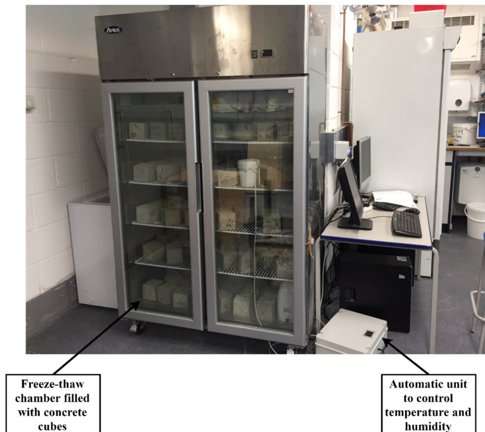
Figure 3-8 - Concrete inside a controlled freeze-thaw chamber
