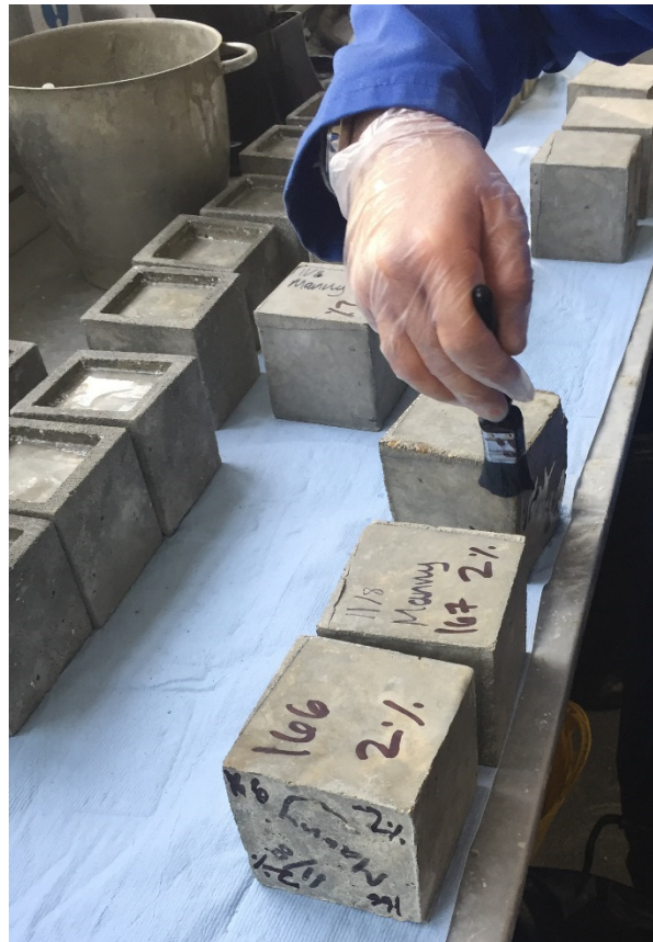
Figure 3-1 - The process of treating concrete with surface impregnations
