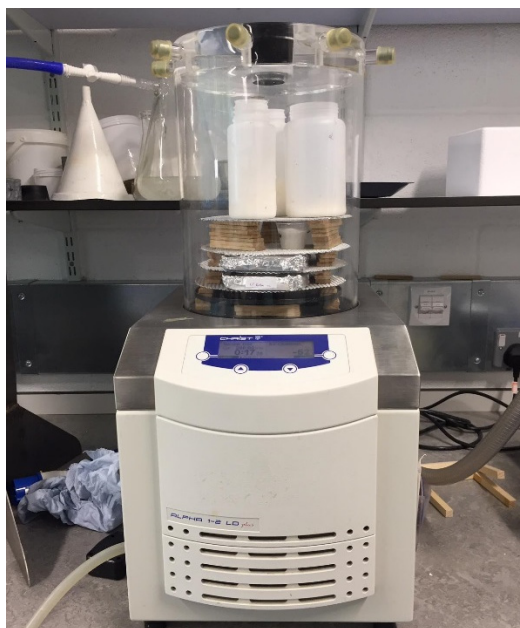
Figure 3-16 - Freeze-drying process of liquid protective materials
