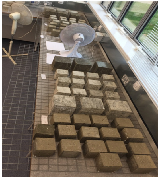
Figure 3-2 - Concrete curing under forced air
