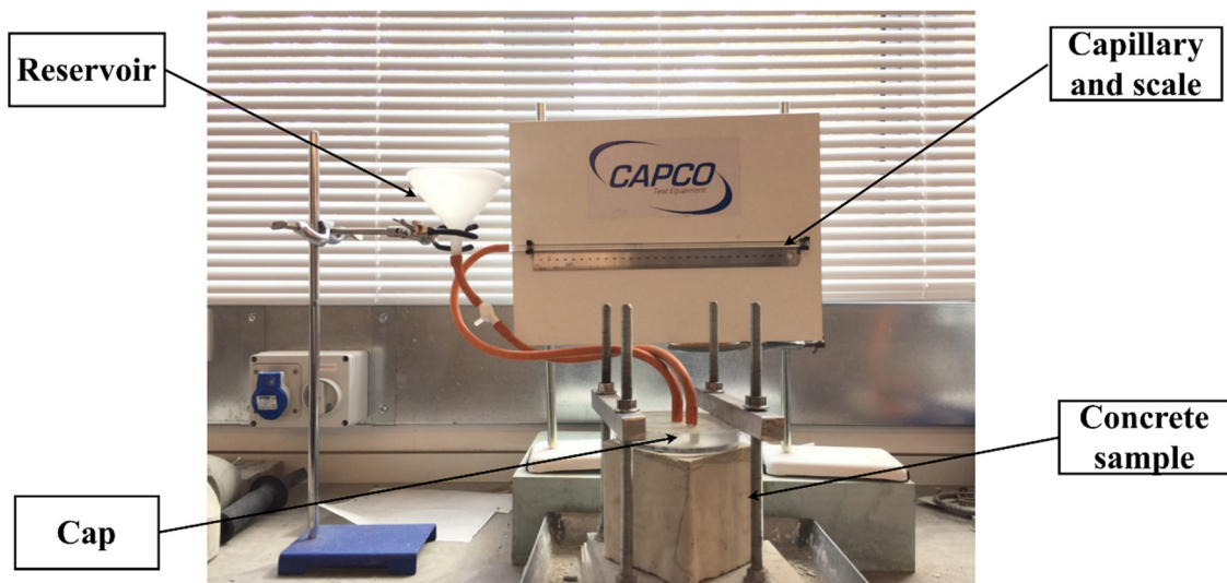
Figure 3-4 – Testing concrete for water absorption with the ISAT apparatus
