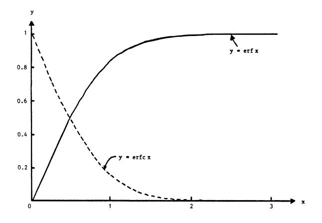
FIGURE 1 Graphs of y = erf x (equation 2.1) and y = erfc x (equation 2.2)
