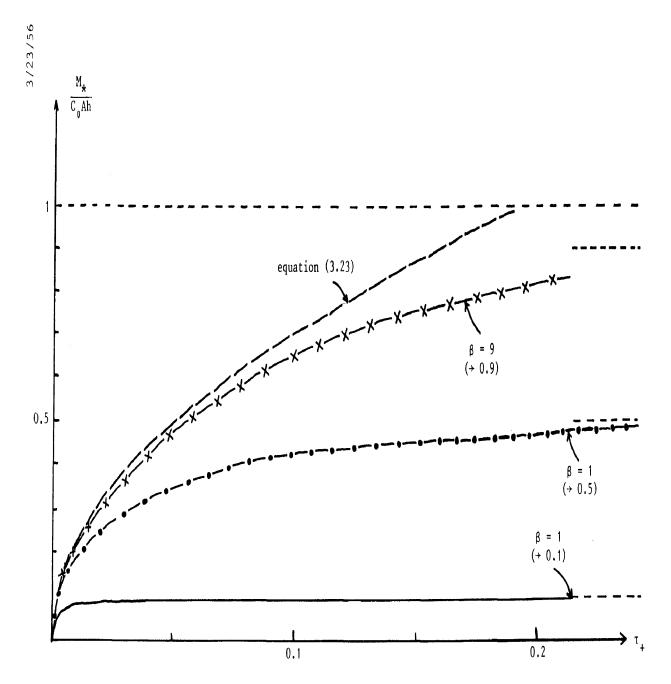
FIGURE 9. The behaviour of  $M_*/(C_0Ah)$  predicted by (3.26) for 3 values of  $\beta$ , where  $\tau_+$  and  $\beta$  are defined in (3.22) and (3.25) respectively. Note that  $M_{*\infty}$  in (3.26) is equal to  $C_0Ah/(1+\beta^{-1})$  - see (3.24). Also shown is the approximate behaviour predicted by (3.23); evidently the accuracy of this approximation depends on  $\beta$  (as well as  $\tau_+$ ).
