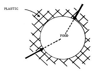
FIGURE 3. Sketch of geometry for second problem of §2.3. Diffusion takes place at <u>each</u> place in the plastic in the direction passing through the centre of the sphere (as indicated by the arrowed lines). The boundary conditions have not yet been discussed. It will be supposed in this example that the interface at x = -a is impermeable to contaminant and that, for large positive x, C(x,t) is close to its initial value  $C_0$ , i.e.
