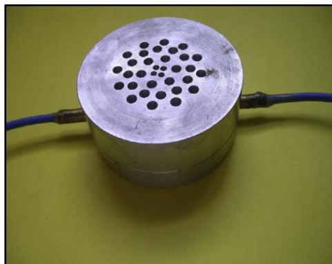
Figure 2.19 Fibre optic hydraulic pressure sensors (Gao, Guo and Liu, 2015)
