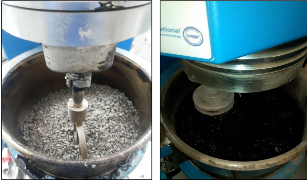
Figure 3.25 Mixing of asphalt material
