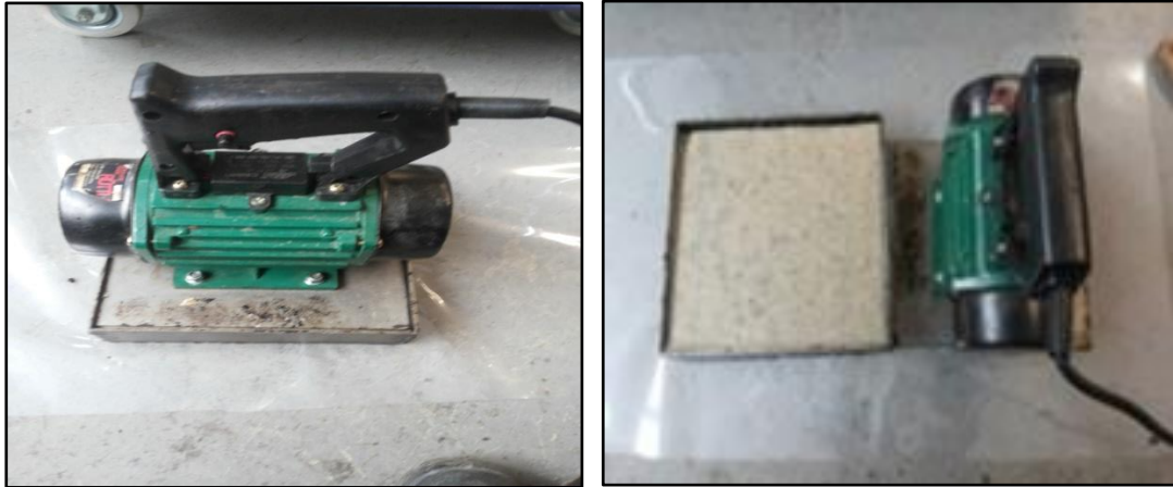
Figure 3.27 Slabs and hand held vibrating plate
