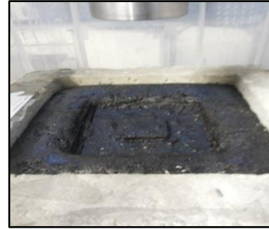
a) Missing aggregate on OPEN SMA surfaces
