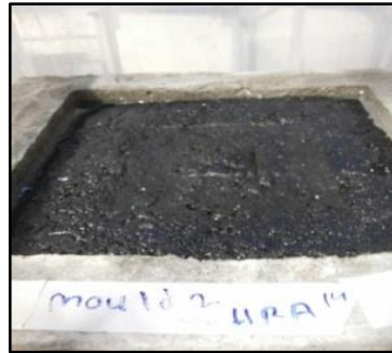
a) Missing aggregate on OPEN SMA surfaces
