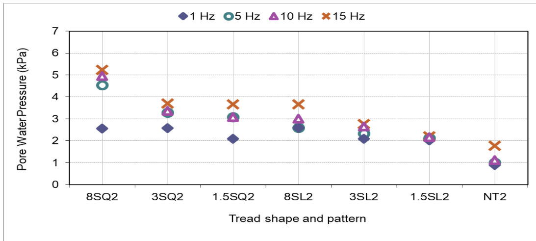
Figure 4.17 2mm surface water, 10kN load, with 20mm asphalt surface
