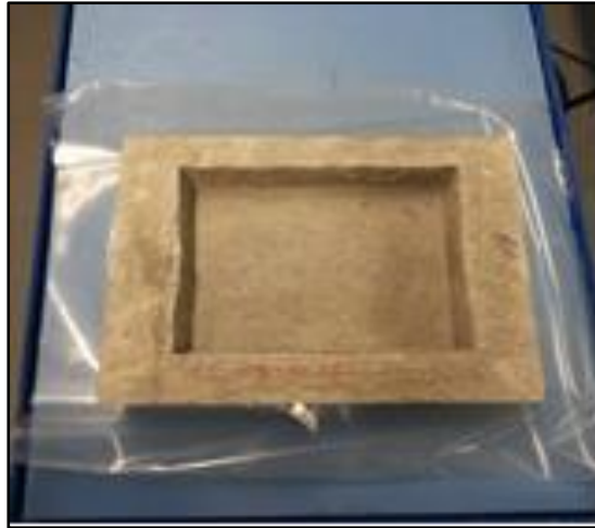
Figure 3.17 Manufactured concrete base
