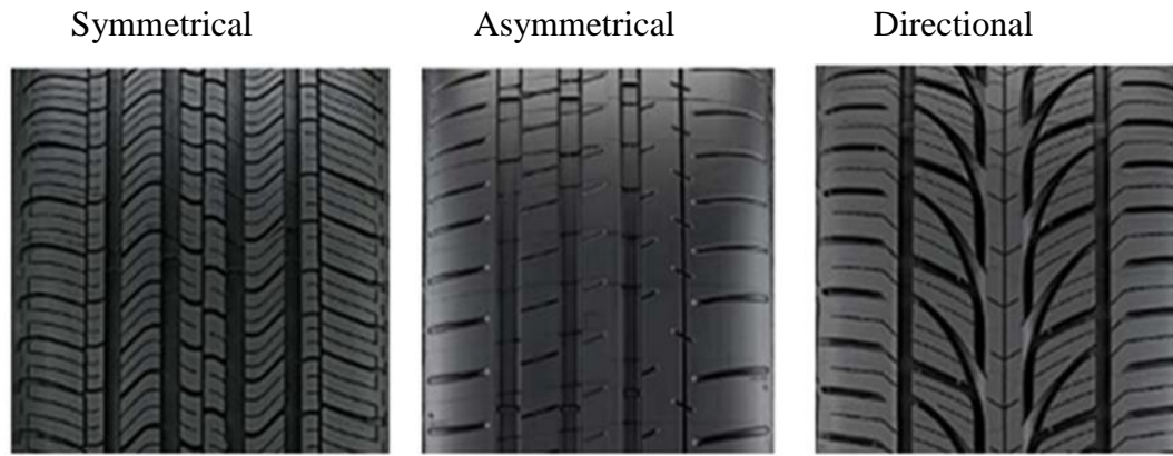
Figure 2.12 Types of tread pattern
