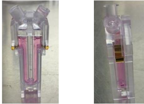
*Figure 3.12: Zeta potential cuvette*
