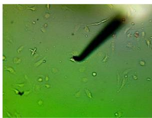
(f) Tip of microelectrode, magnification  $\times 200$
