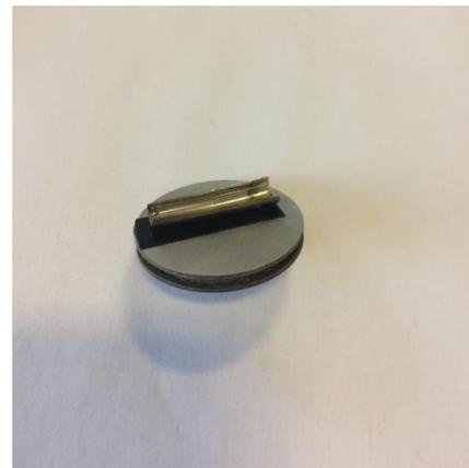
(e) Mounting the specimen on an aluminum pin stub
