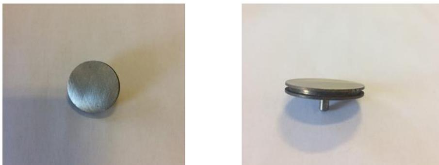
*(a) An aluminium pin stub*
