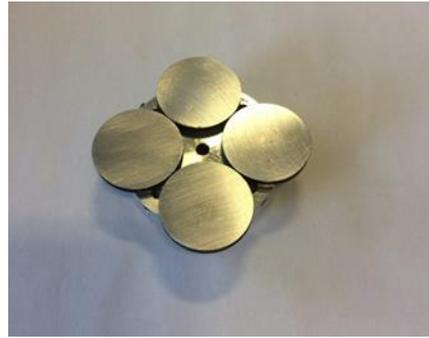
(c) Four aluminum pin stubs placing on a multi-pin stub holder
