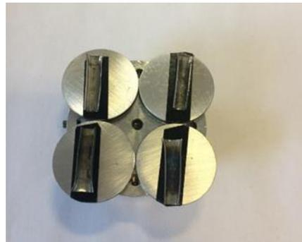
(f) Prepared specimens to use in a sputter coating system and scanning electron microscopy
