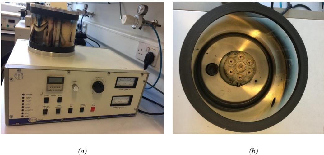
Figure3.40: The sputter coating system (a) and the chamber of sputter coating system (b)
