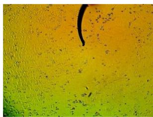
(e) Tip of microelectrode, magnification  $\times 80$
