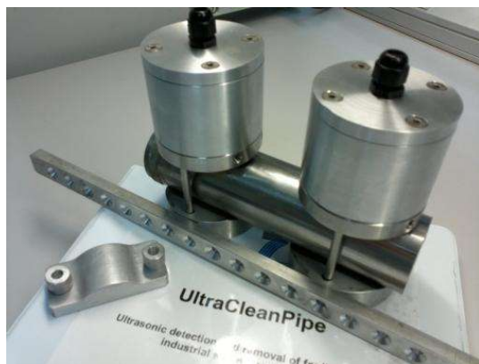
Figure A.4. Assembly with the transducers aligned by the ruler.
