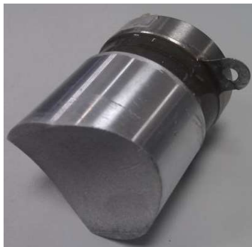
Figure A.6. UCP transducer
