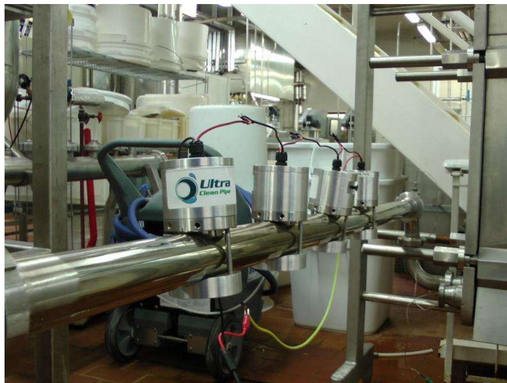
Figure 8.18. UltraCleanPipe transducers and support attached for the field trials. Flow of 230 l/min.
