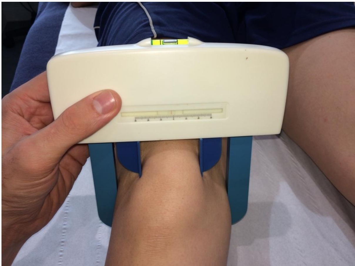
Figure 4.3. The Patellofemoral Calliper measuring the offset between the patella centre and transepicondylar centre.
