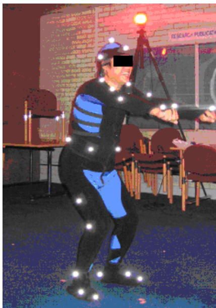
Fig 1 Motion Capture by Eagle Digital System Using Helen Hayes Marker Set
