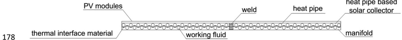
179 Figure 1: Cross Section of the Heat Pipe Based PV/T Panel [30]
