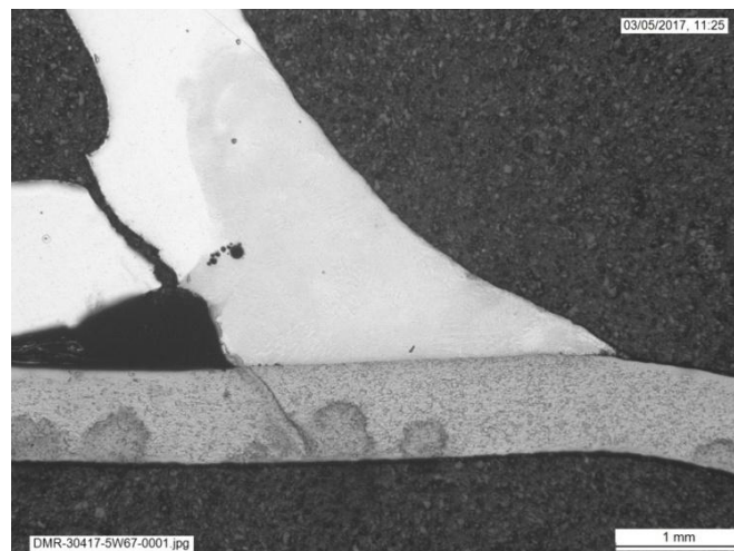
Figure 4.44) Image of tensile shear specimen after testing, B6
