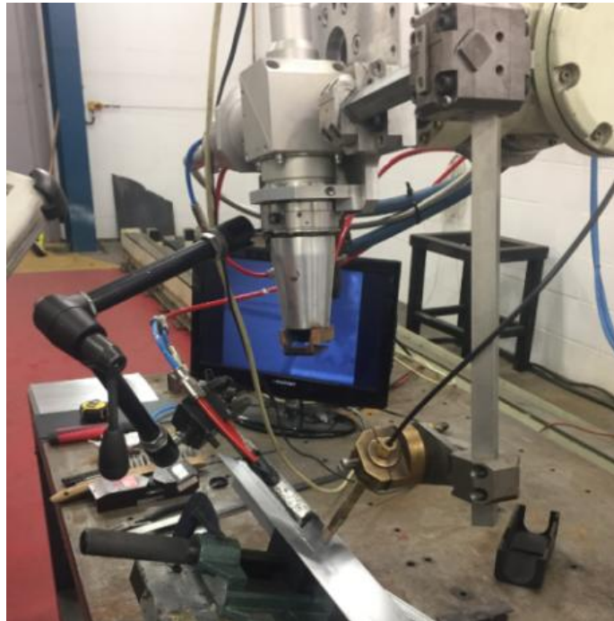
Figure 3.4) Image of the experimental laser brazing set-up used in brazing trials
