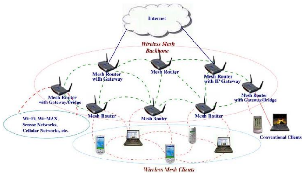
Figure 2.4 WMNs hybrid architecture [1]
