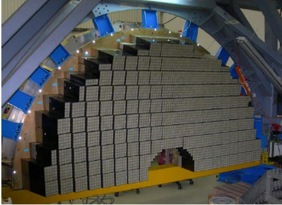
Figure 2-7 – An endcap Dee, showing the supercrystals and individual lead tungstate crystals within each supercrystal [15].
