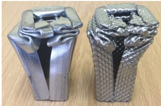
Fig. 12. Asymmetrically crushed specimens due to inherent imperfection
