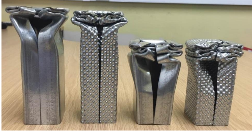
Fig. 13. Typical deformed shapes of tested specimens
