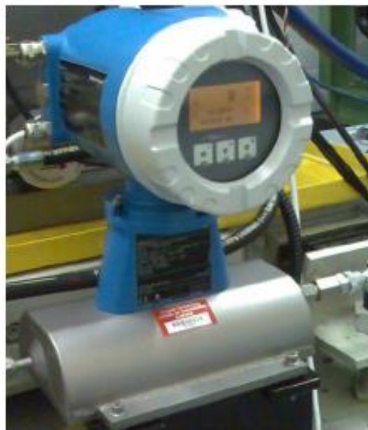
Figure 3-5 Coriolis mass flow meter by Endress+Hauser
