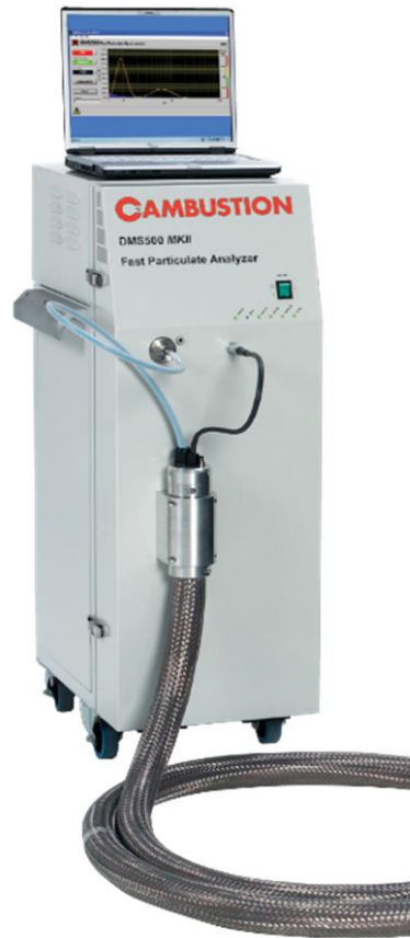
Figure 3-26 Cambustion DMS 500 fast response particulate analyzer
