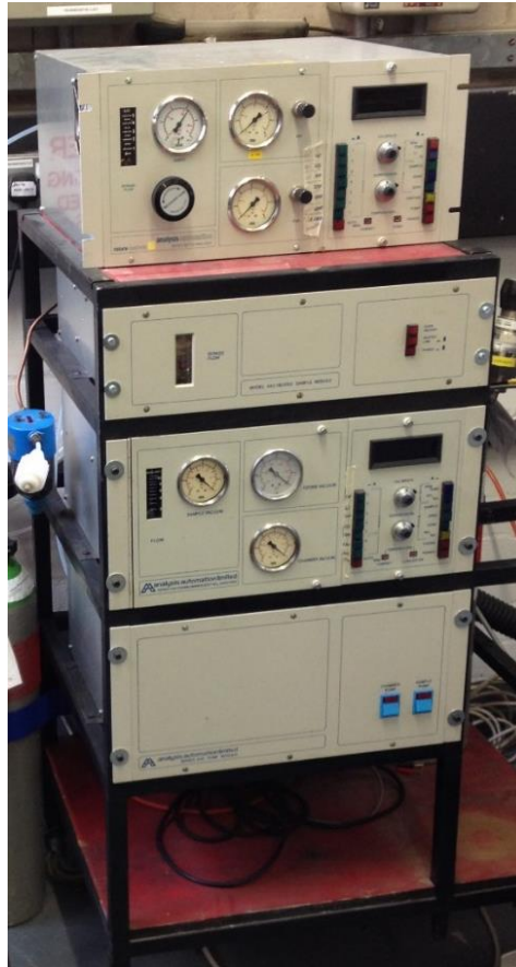
Figure 3-24 Signal Rotork Analysis model 523 FID analyser used for HC measurements (first unit at the top) and Signal Ambitech model 443 Chemiluminescent analyser used for NO/NO x measurements (bottom three units)
