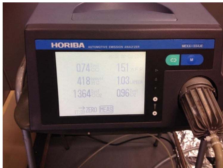
Figure 3-23 Horiba MEXA-554JE for CO, CO 2 and O 2 measurements
