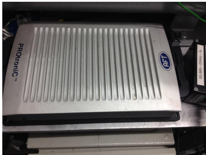
Figure 3-13 Mahle Flexible engine control unit
