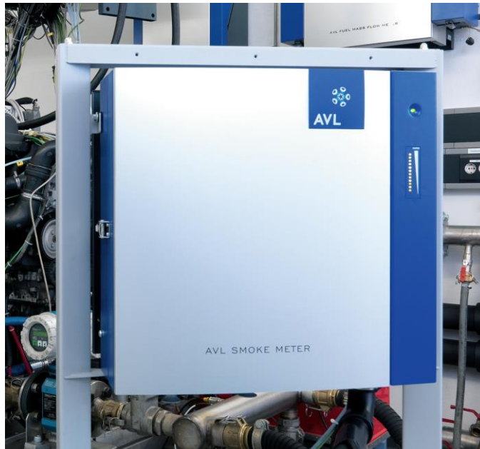
Figure 3-25 AVL 415SE smoke meter used for particle measurement
