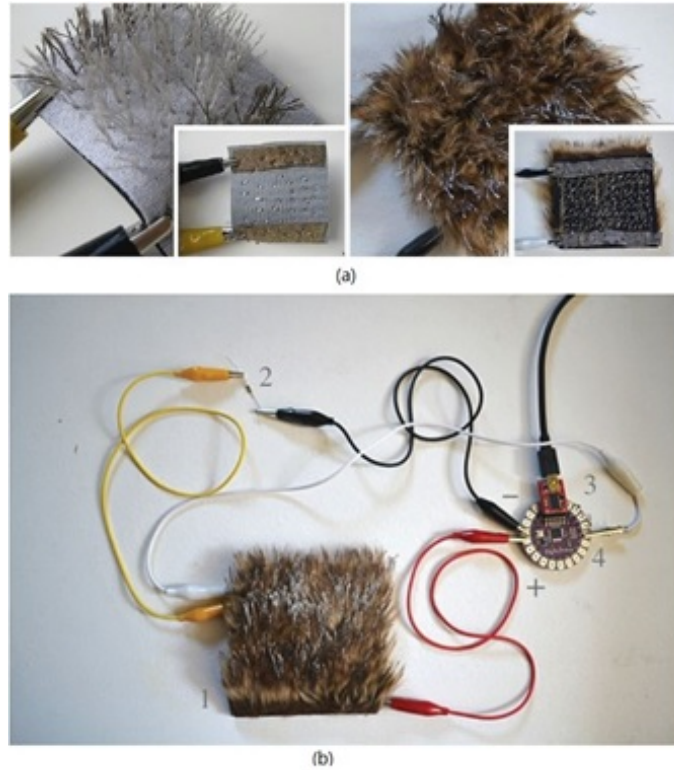
Figure 3.1: Pictures of the conductive fur sensor, (a) is basic look of conductive fur touch and gesture sensor and (b) is basic construction of fur sensor prototype [3]
