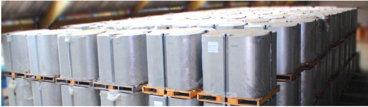
Figure 1.5: Intermediate nuclear waste container made of grade 2205 DSS Courtesy of Graham Engineering, BB9 8SY Nelson, UK
