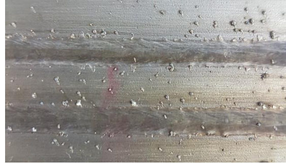
Figure 5.15: Heavy spatter caused by dual beam
