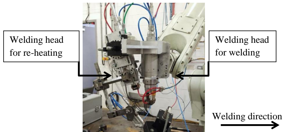
Figure 5.1: Dual beam set up
