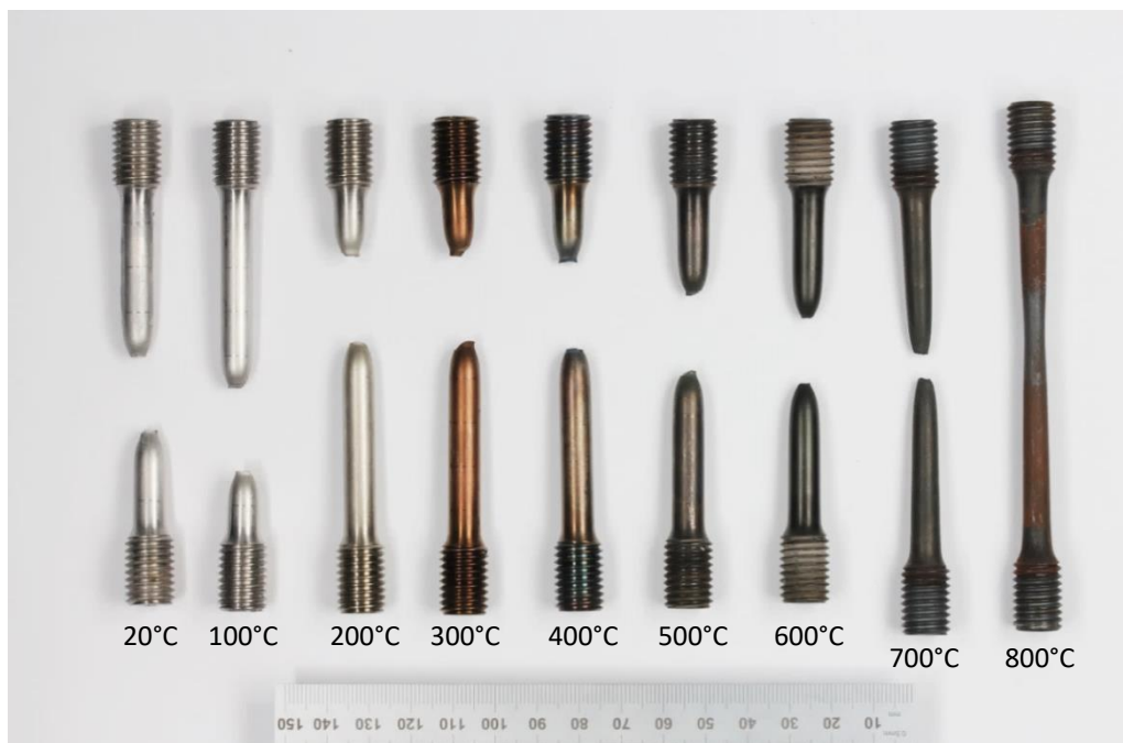
Figure 4-3 Steel A (S690QL) tensile specimens after isothermal tensile tests at various elevated temperatures
