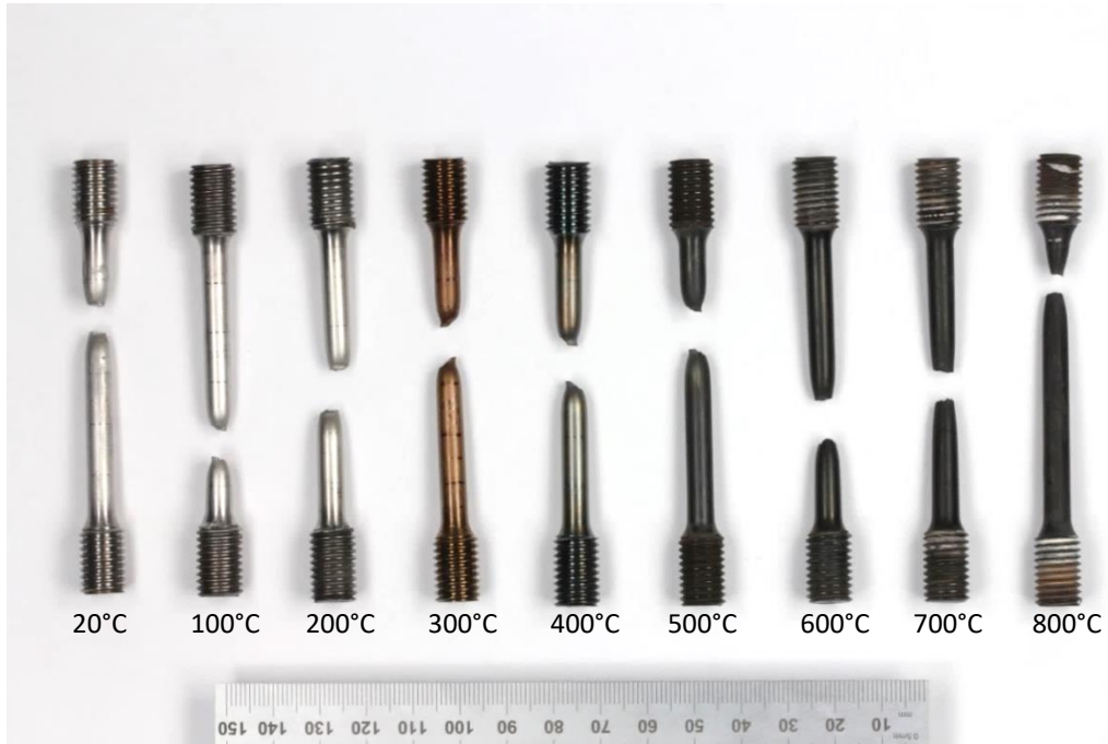
Figure 4-4 Steel B (S700MC) tensile specimens after isothermal tensile tests at various elevated temperatures
