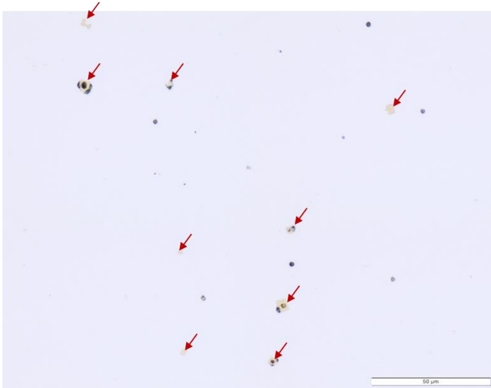
Figure 5-12 Light microscope of steel B (S700MC) - unetched
