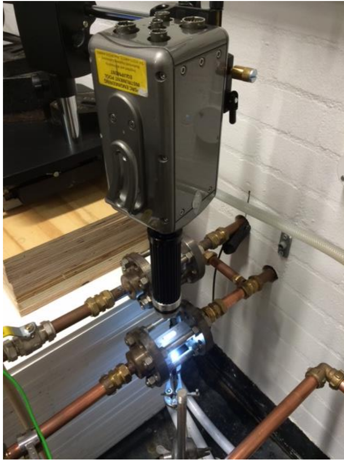
Figure 3. 12 Phantom V5.1 Digital High-Speed Camera
