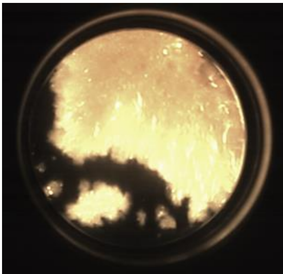
Figure 6-10 Blown-up view of the multiple auto-ignition initiation sites observed during the tests
