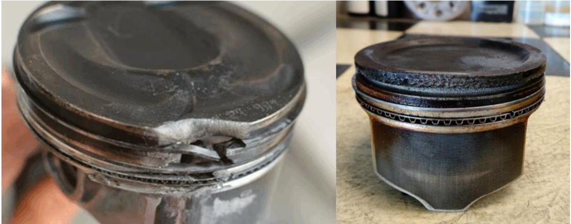
Figure 2-20: : Samples of knock damage to piston rings and piston crown [108].
