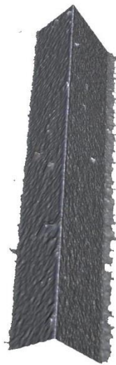
Figure 6-7 PCD end mill surface morphology of new and used tools
