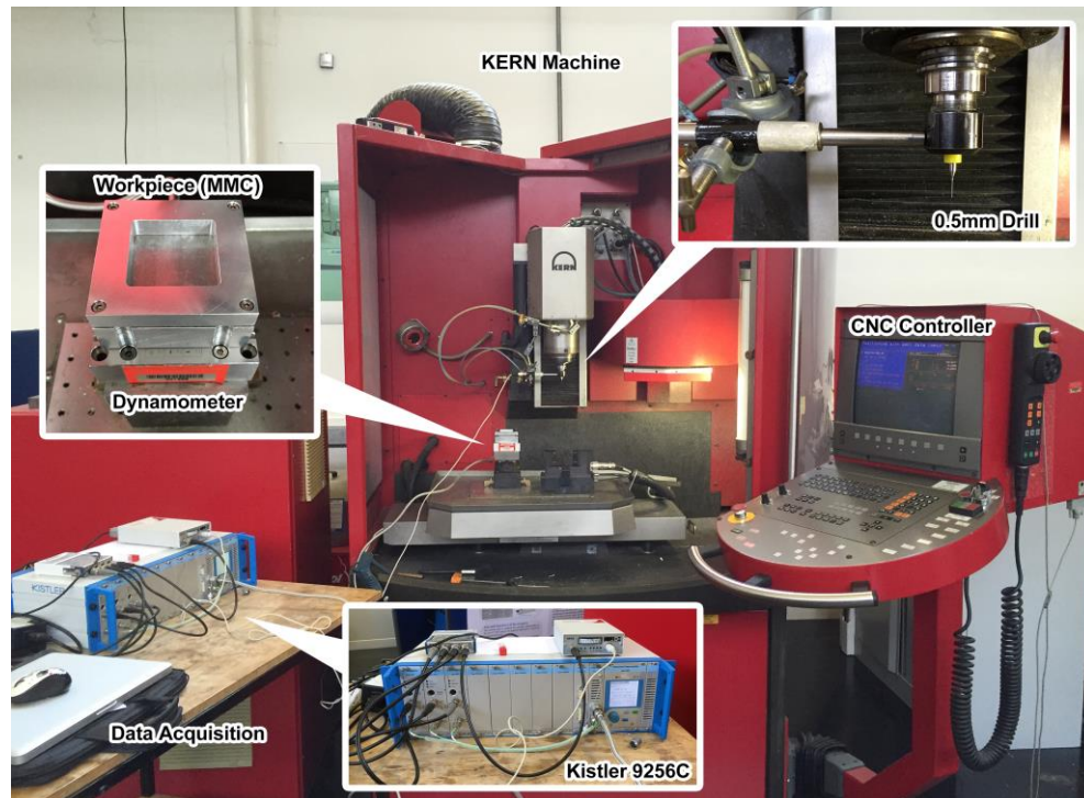
Figure 2 Micro drilling experimental set-up
