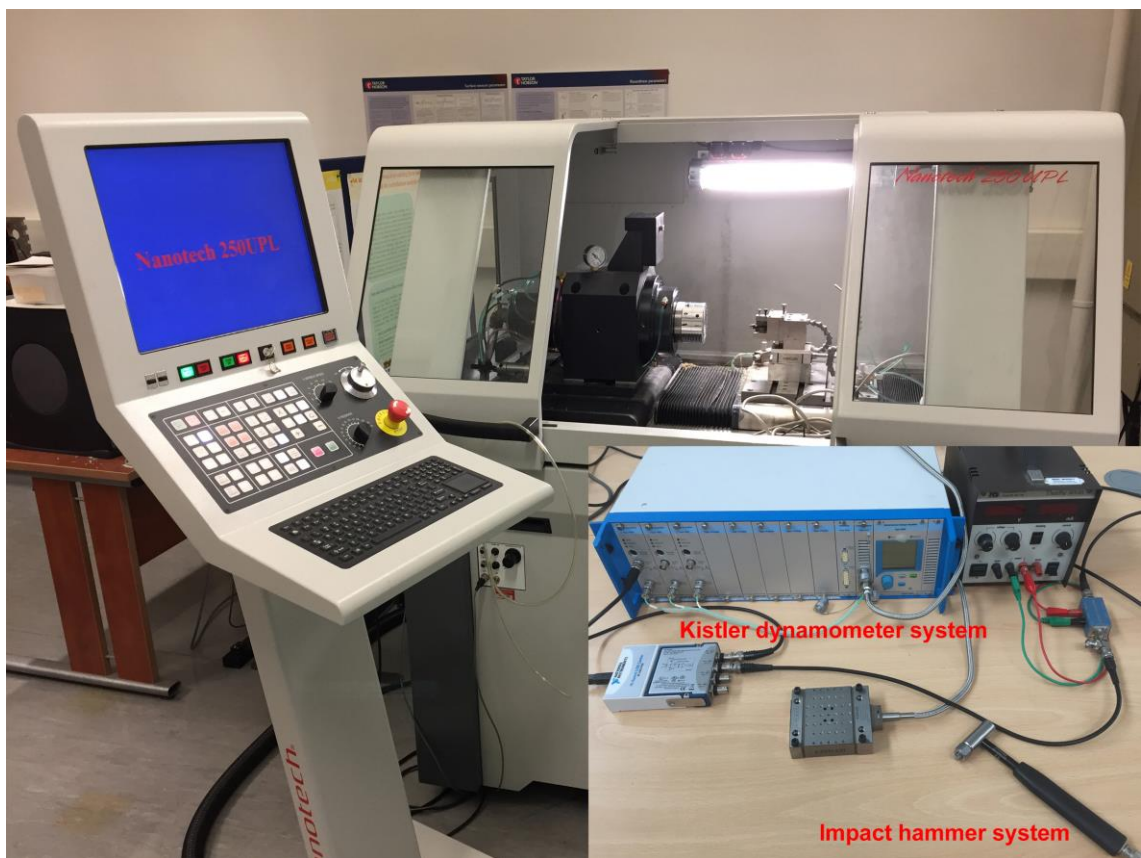
Figure 3-4 Precision turning experimental set-up
