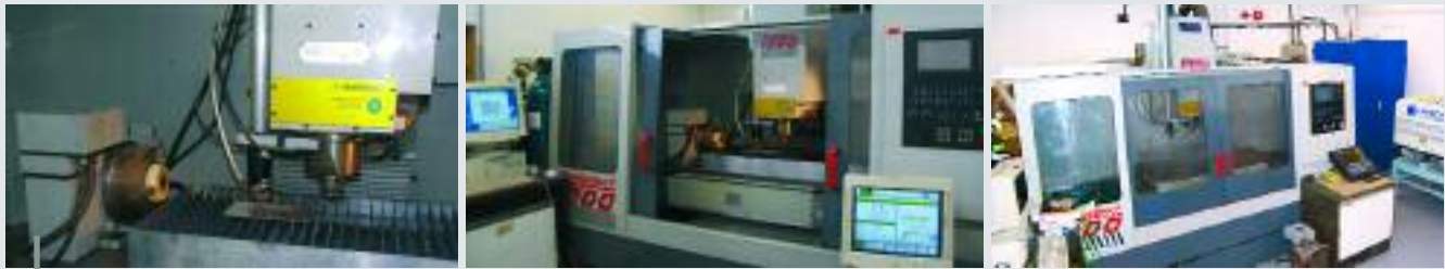
Trumpf TLF1200W laser. The beam is enclosed within tubes but bounces off a series of mirrors into a 4 axis Bridgeport CNC machining center
