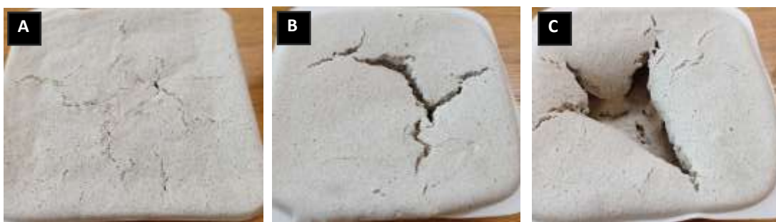
FIGURE 4.3 DIFFERENT DEGREE OF CRACKING IN THE DRY FOAMS A) MINOR B) MEDIUM AND C) SEVERE
