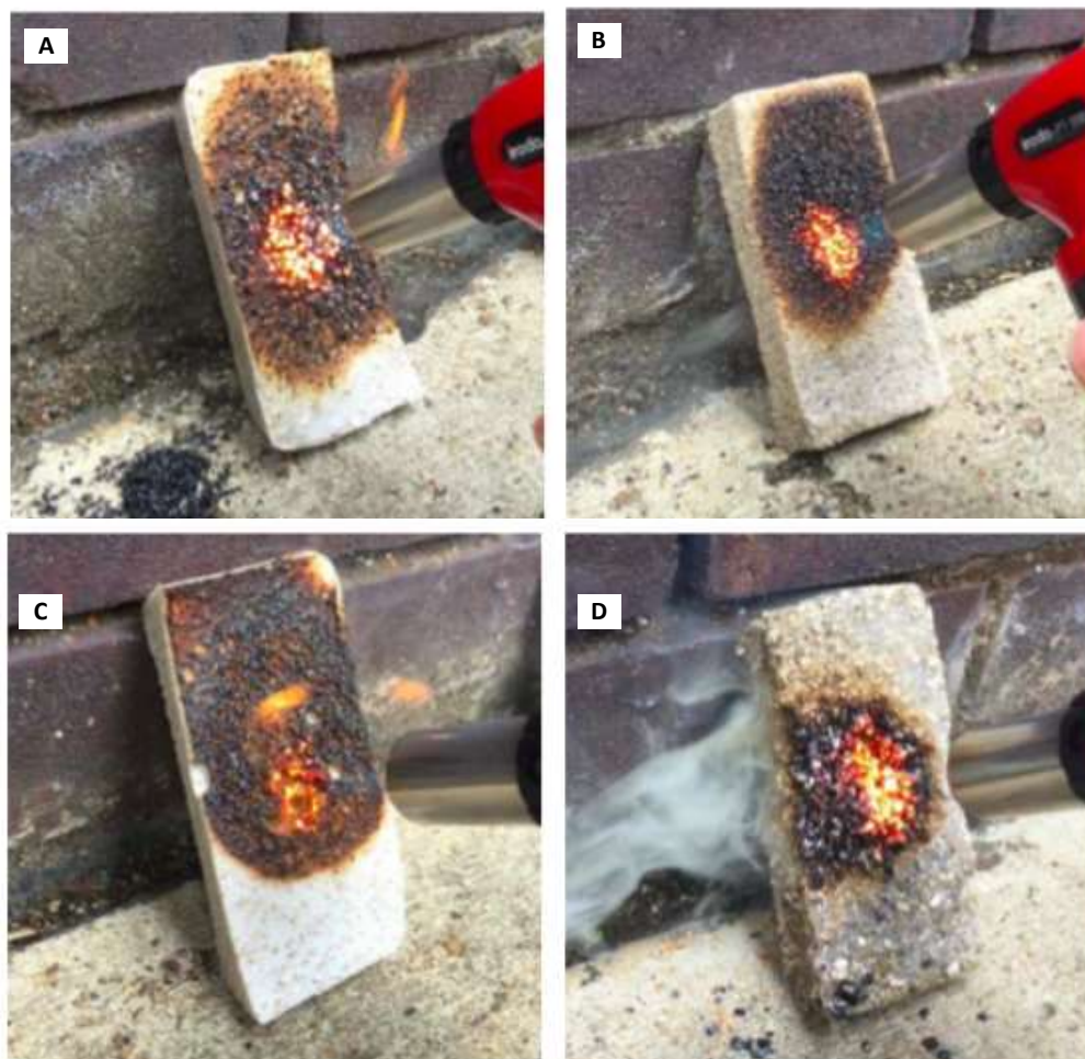
Figure 6.18. RESPONSE OF THE GELATINE VERMICULITE COMPOSITE FOAMS TO DIRECT FLAME EXPOSURE FOR 15 SECONDS: (A) SAMPLE VB9; 20 wt% GELATINE, 19.5VOL% COARSE VERMICULITE (B) SAMPLE VS9; 20 wt% GELATINE, 19.5 VOL% FINE VERMICULITE (C) SAMPLE VS3; 20 wt% GELATINE CONTENT, 6.5 VOL% FINE VERMICULITE (D) SAMPLE VB7; 10 wt% GELATINE CONTENT, 6.5 VOL% COARSE VERMICULITE
