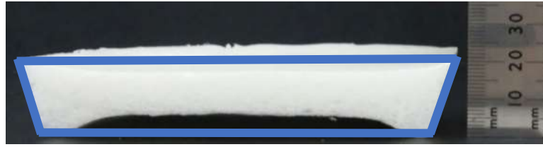
Figure 4.5. TYPICAL CROSS-SECTION TO ALL THE CASTS OF STARCH-GELATINE FOAMS SHOWING THE SHRINKAGE FROM THE MOULD OUTLINED AND FREE OF DEFECTS.
