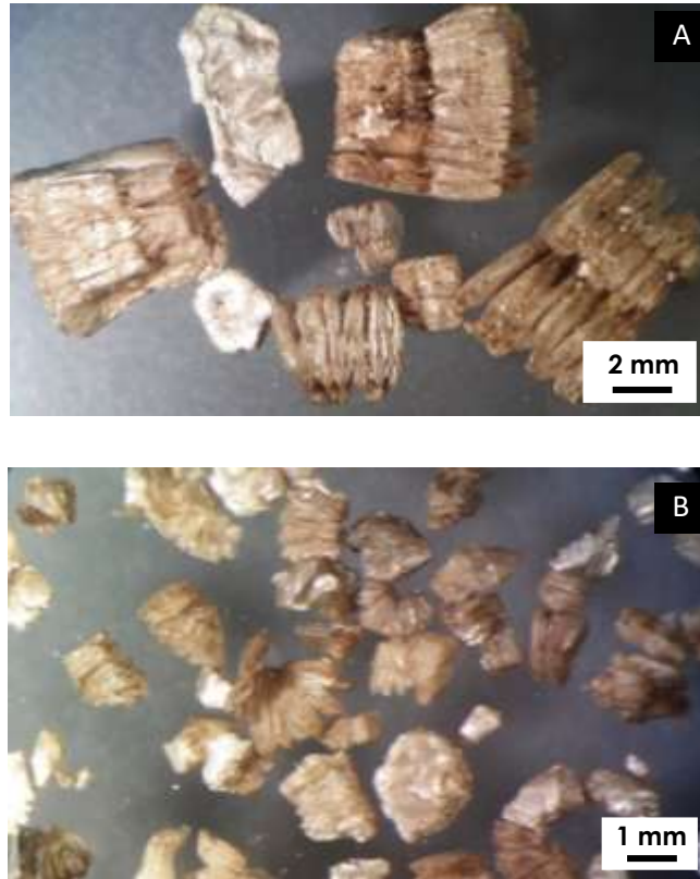
Figure 3.8. OPTICAL MICROSCOPE IMAGES OF THE EXPANDED VERMICULITE PARTICLES (A) COARSE VERMICULITE (B) FINE VERMICULITE
