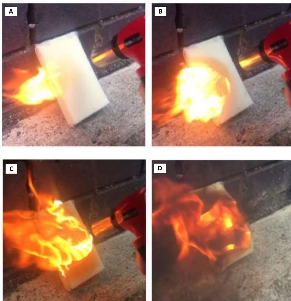
Figure 6.15. RESPONSE OF POLYURETHANE FOAM IN DIRECT FLAME EXPOSURE (1300°C) FOR THE LENGTH OF TIME (SECONDS) (A) 1 (B) 3 AND (C) 10
