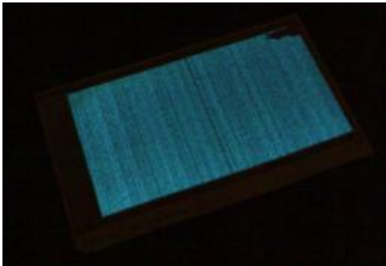
Fig. 1.4 Offset lithographically printed electroluminescent display. The array has 100 \mu\text{m} track and gap spacings producing a field of 2 \times 10^6 V/m 2 at an operating voltage of 200 V [21].
