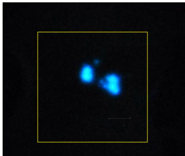
Fig. 6.5 A structure of 25 \mu\text{m} track and gap stimulated with a driving voltage of 65 V. The total device area of 3 mm x 3 mm is bound by the yellow box.
