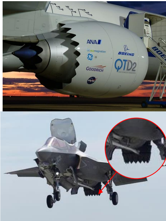
Figure 1.1. Boeing 787 (top) and F-35B (bottom) engine/nozzle with chevrons for noise reduction
