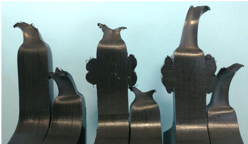
Figure 4-15 image of the high speed tensile impact specimens illustrating the difference in deformation left to right: unwelded parent material specimen (Parent), typical welded specimen (WP1-3C), and high deformation welded specimen (WP5-3A)
