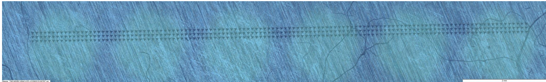
Figure G-7 Microscopy image of WP2 post-nanoindentation showing the full 120 indent grid, Olympus BX41 LED at 2.5X resolution
