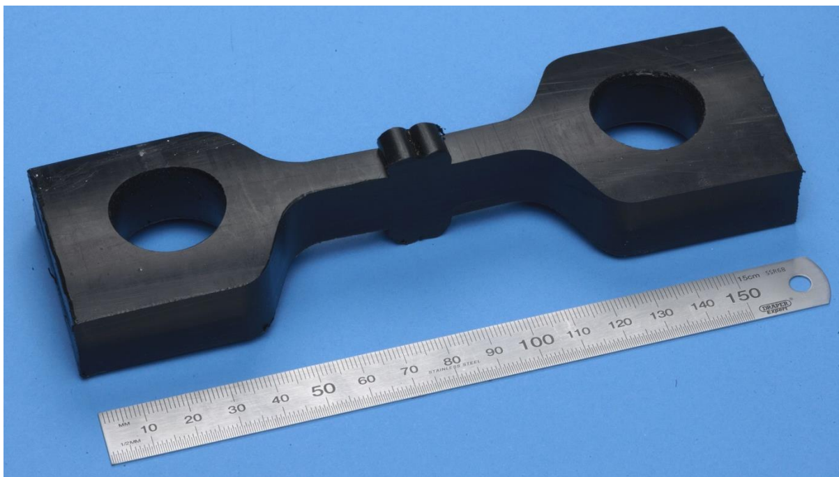
Figure 4-11 High speed tensile impact test specimen (not actual specimen) (TWI, 2016)
