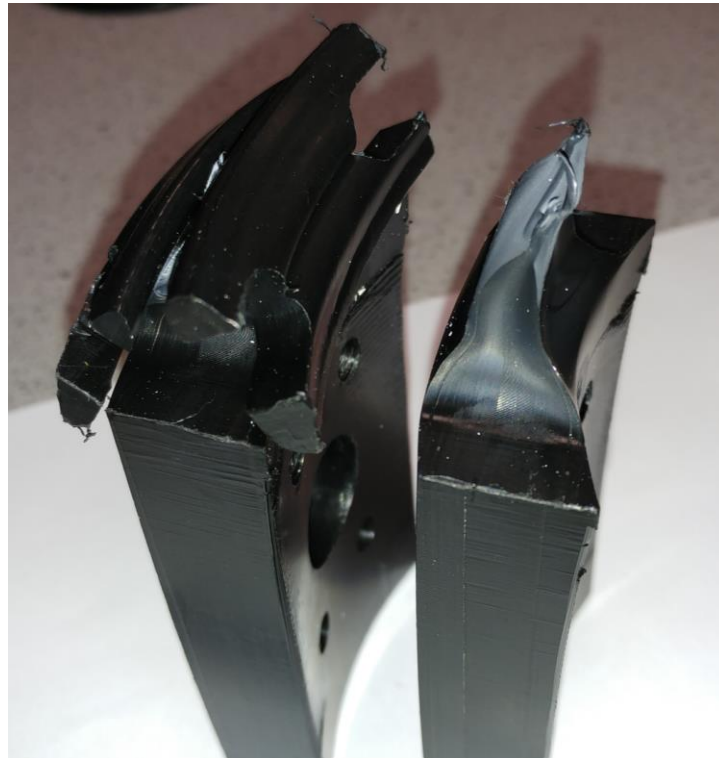
Figure 4-5 Image of the failure in a typical waisted tensile test specimen featuring ductile fracture surfaces at the weld
