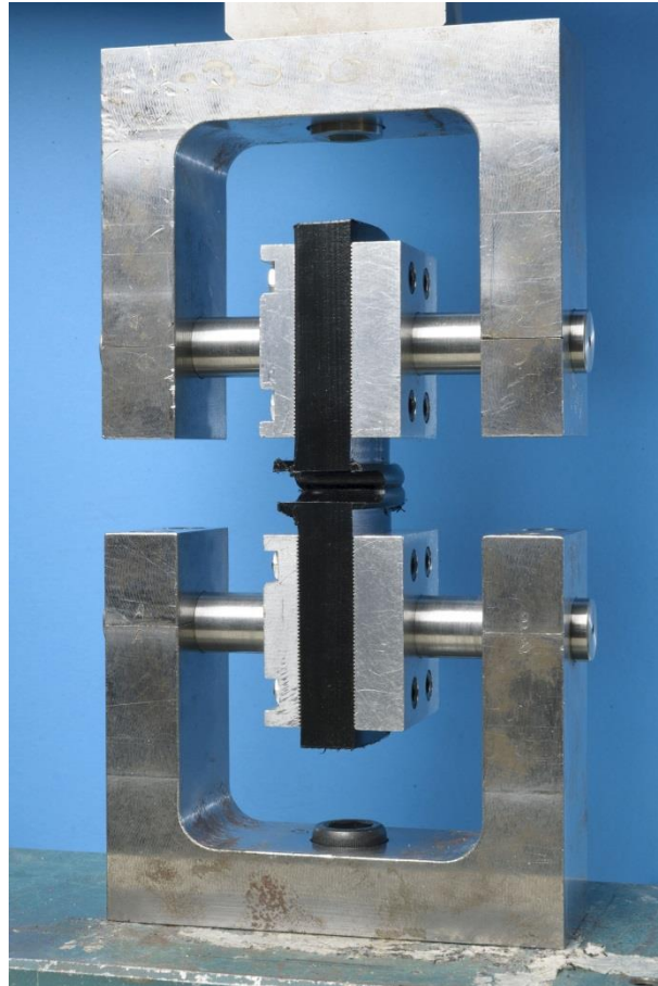
Figure 4-4 Waisted tensile test specimen set-up inside the testing jig (TWI, 2016)
