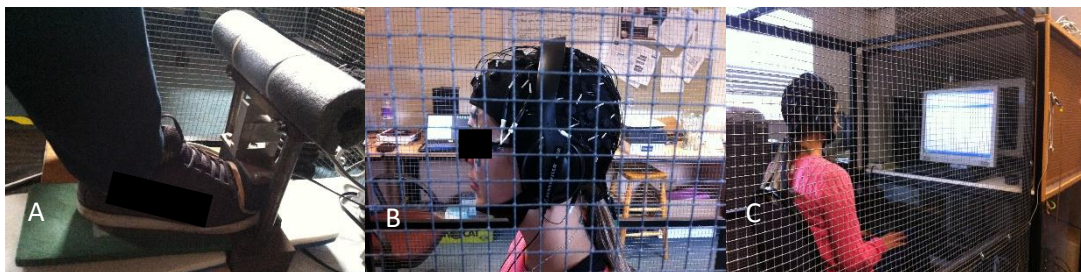
Figure 3.1. Experimental set-up of Study 1. Figure 3.1A: Force transducer used to quantify the level of pressure generated by the participant against the load cell; Figure 3.1B: Participant wearing the EEG cap and headphone; Figure 3.1C: Participant's vision from outside the Faraday cage; the cage was assembled to prevent the electrical interference of external devices.
