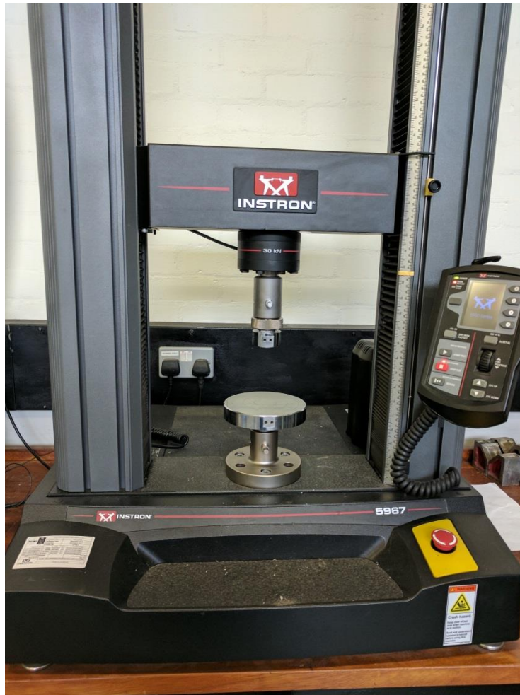
Figure 4-5 Compression machine used to carry out stress-strain tests
