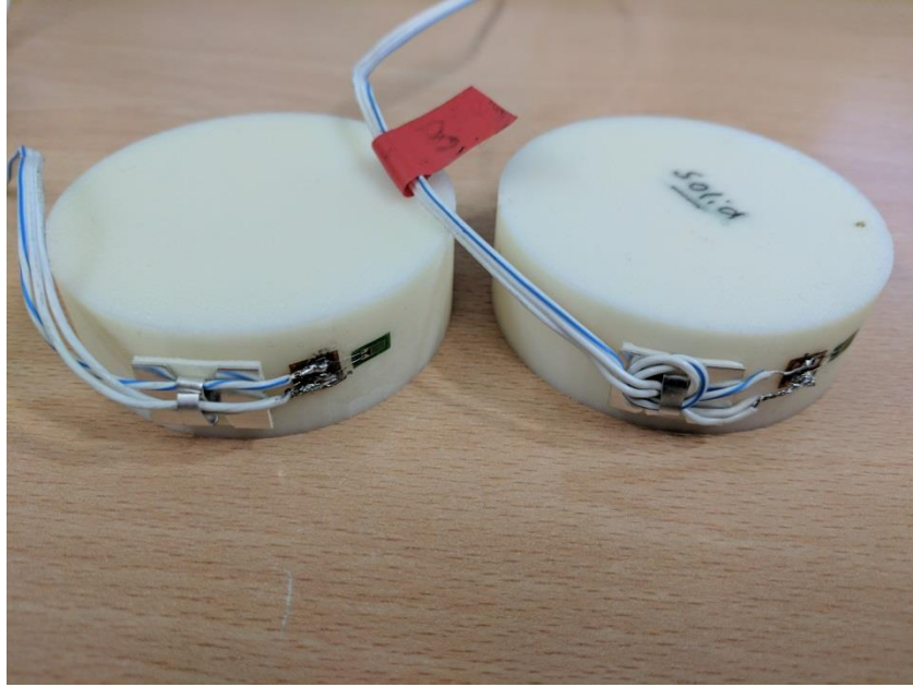
Figure 4-6 ABS models of solid and hollow shell cylinders
