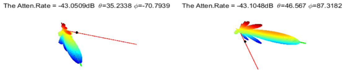
Figure 5- 28: The beams in the 16×16 antenna arrays system with 2 beams
