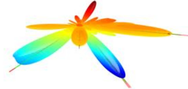
Figure 5- 4: The 3D beam in the 16×16 antenna arrays system with 4 beams
