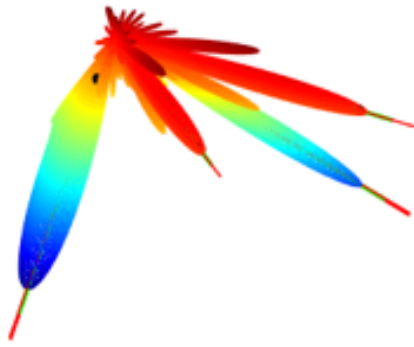
Figure 5- 21: The 3D beam in the 32×32 antenna arrays system with 4 beams
