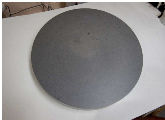
Figure 3.11: The Lithium Hydride disk absorber. Radius 225mm, thickness 65mm. [7]
