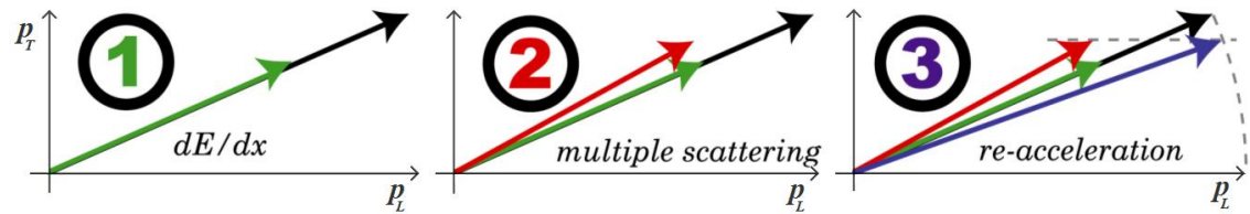
Figure 3.2: Graphical representation of emittance reduction. In the first figure, the overall momentum vector of the muon is reduced. Then the heating effect of scattering is considered, which increases the transverse component of the momentum vector. Finally, the beam is accelerated in the longitudinal direction. Overall, the transverse momentum is reduced and the proaxial momentum is maintained.
