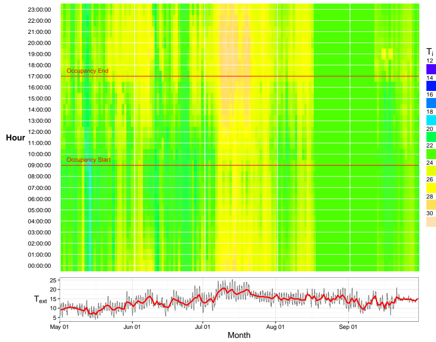
FIGURE 4.1: Heat-map of indoor air temperature in open plan office B294 (taken as operative temperature as discussed earlier)
