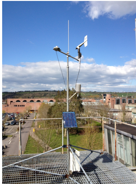
FIGURE 3.17: Roof mounted weather station with recommissioned Campbell Scientific instrumentation. See Table 3.7 for instrument specifications
