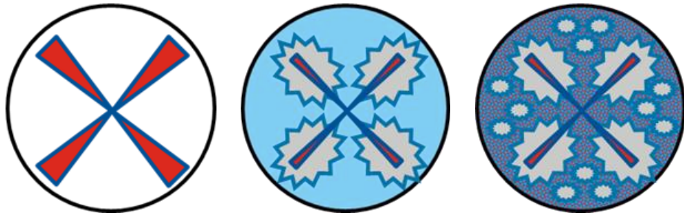
Figure 5-1: Proposed visual depiction of the three different combustion modes tested: Diesel (left), Conventional Dual-Fuel (middle), and PDFC (right).
