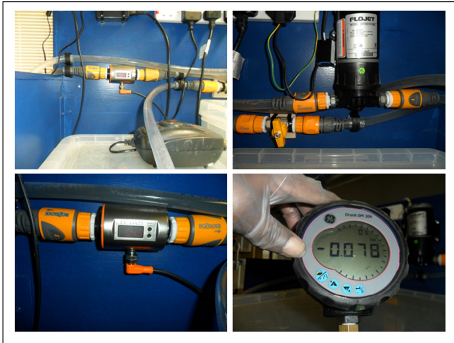
Figure AP.B.2. (Left) – SMBR rig flow meter being used; (Right) – Diaphragm pump and a pressure gauge in operation
