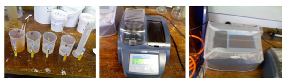
Figure 3.10. Pictures of a COD test to be carried out. 2 mL of each sample solution is pipetted respectively into a cuvette. The HACH is then used to conduct the test and finally COD is measured with the DR 900. Images from left to right are sample solutions, HACH device and DR 900 measurement kit
