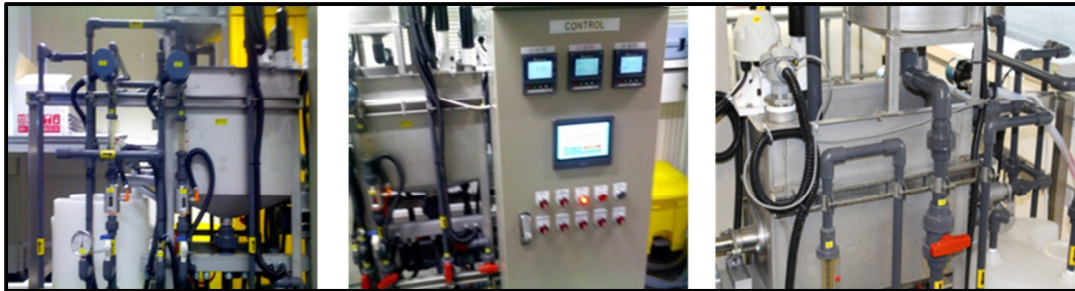
Figure 3.1. Set-up pictures of the RPU-185 RMBR in operation as the rotating membrane module is located in the batch tank (picture on the right) for filtration purposes. Equipped with a Human-Machine Interface (HMI) touch screen, most of its functionalities are automated
