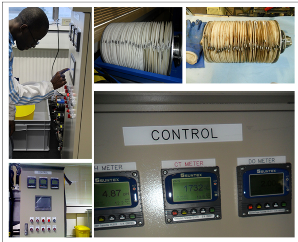
Figure AP.B.1. (Left) – RPU-185 RMBR pilot unit being operated by PhD author; and, below this is an overview of control panel; (Right) – Non-fouled and fouled rotating membrane module; respectively on image below them are: pH, Conductivity and D.O. meter
