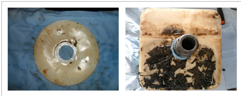
Figure 7.2. (Left) Impact of fouling on the RMBR system - Even caking is observed. (Right) Impact of fouling on the SMBR system - Uneven caking is observed
