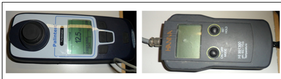
Figure 3.13. (Left) Turbidity read with Palintest turbidity metre. (Right) HANNA H1 991300 conductivity metre
