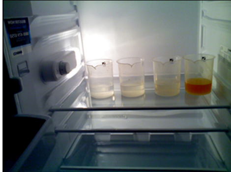
Figure 3.9. Refrigerated chemical solutions (from left to right respectively, \text{NH}_4\text{Cl} , \text{CaCl}_2 , \text{Mg}_2\text{SO}_4 \cdot 7\text{H}_2\text{O} , and \text{FeCl}_3 \cdot 6\text{H}_2\text{O} )
