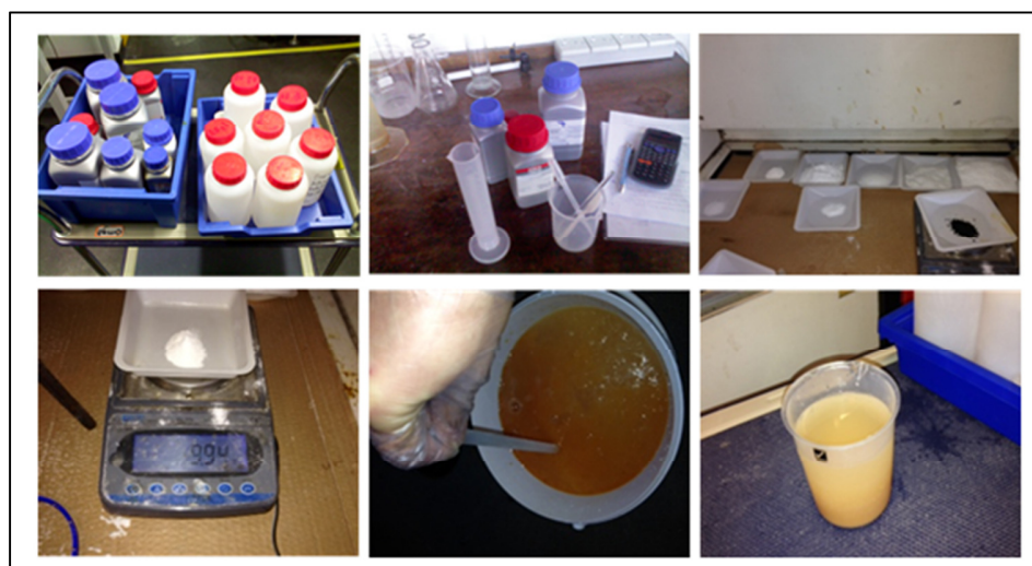
Figure 3.8. Pictures of the production of synthetic wastewater in laboratory. After stirring-up the concentrate, 500 mL of it is poured into a beaker to top-up 500 mL of distilled water, making one litre of synthetic wastewater
