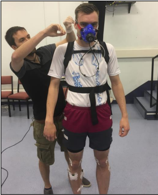
Figure 5.4. Attaching the Cosmed K5 on one of the participants for pulmonary gas collection.
