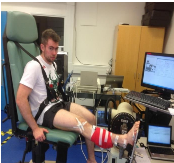
Figure 3.3. Participant on the dynamometer for the assessment of ankle plantarflexors neuromuscular performance.
