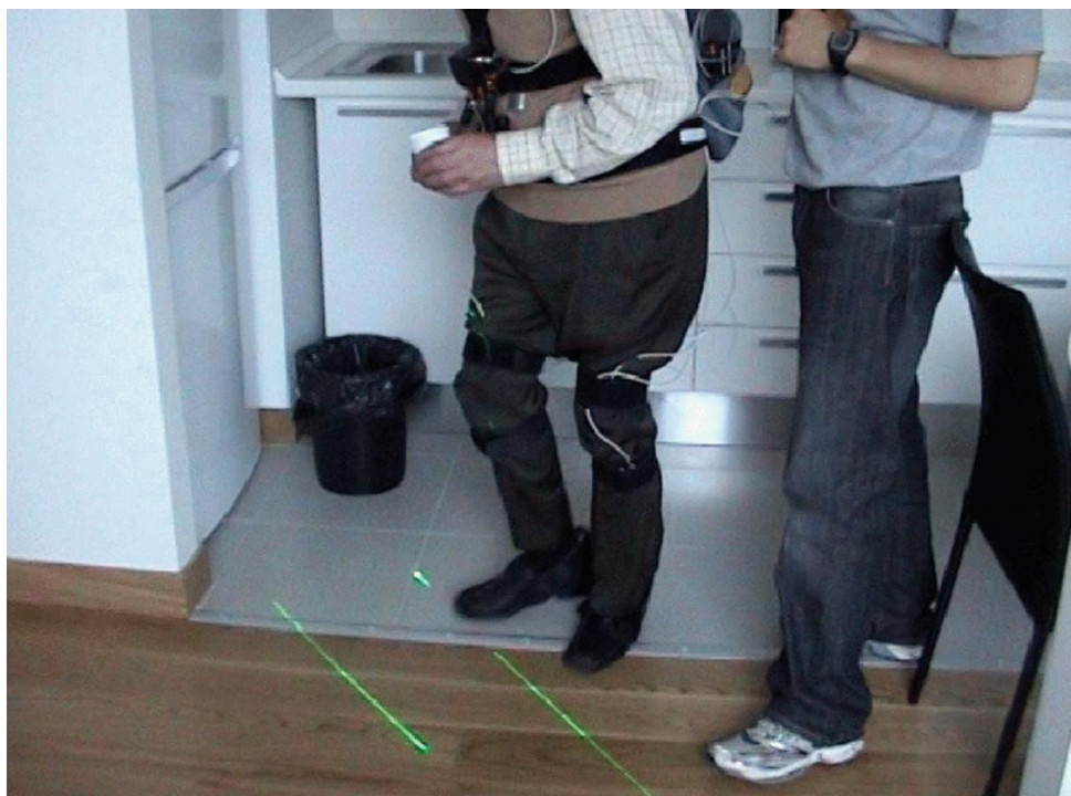
Figure 2:2. A SMLD coupled with a controlling laptop and laser line projection system for PD patient's visual cue purposes [31]
