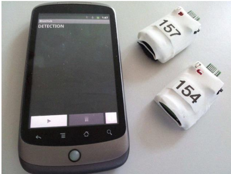
Figure 2:5. A pair of accelerometers and a smart phone used for gait analysis and FOG assessments in PwP [39]
