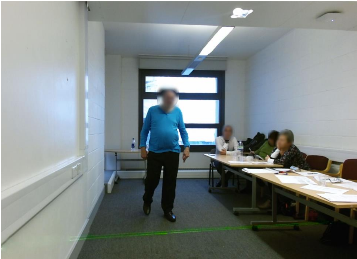
Figure 5:20. A PD patient volunteering to try out the system's capabilities in detecting FOG. Visual cues are projected in front of him, on the floor based on his whereabouts
