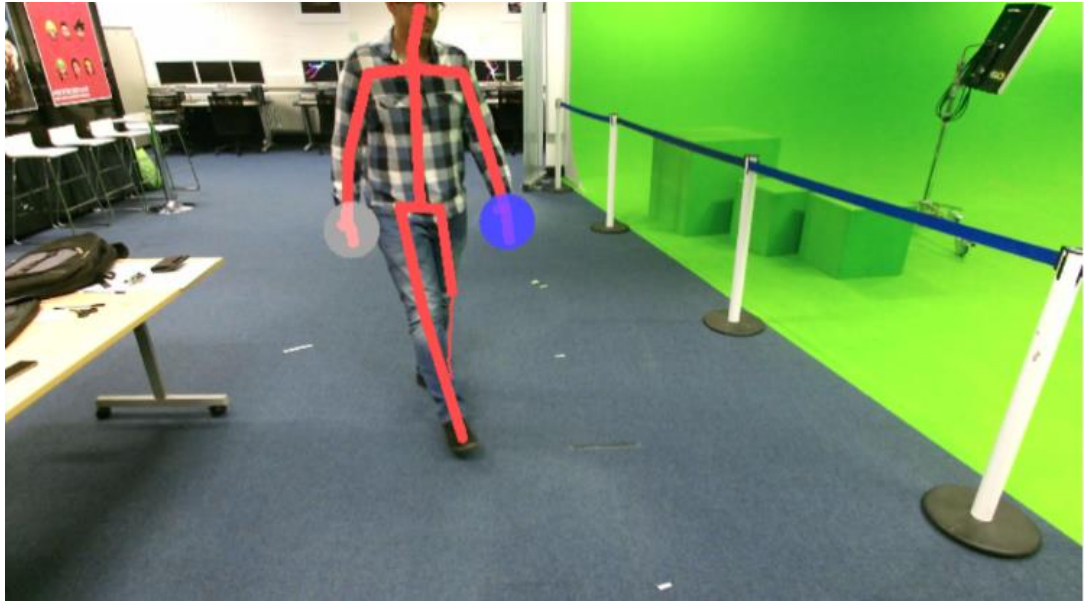
Figure 5:1. The testing environment: the subject is walking diagonally towards the Kinect camera while his body joints are being tracked
