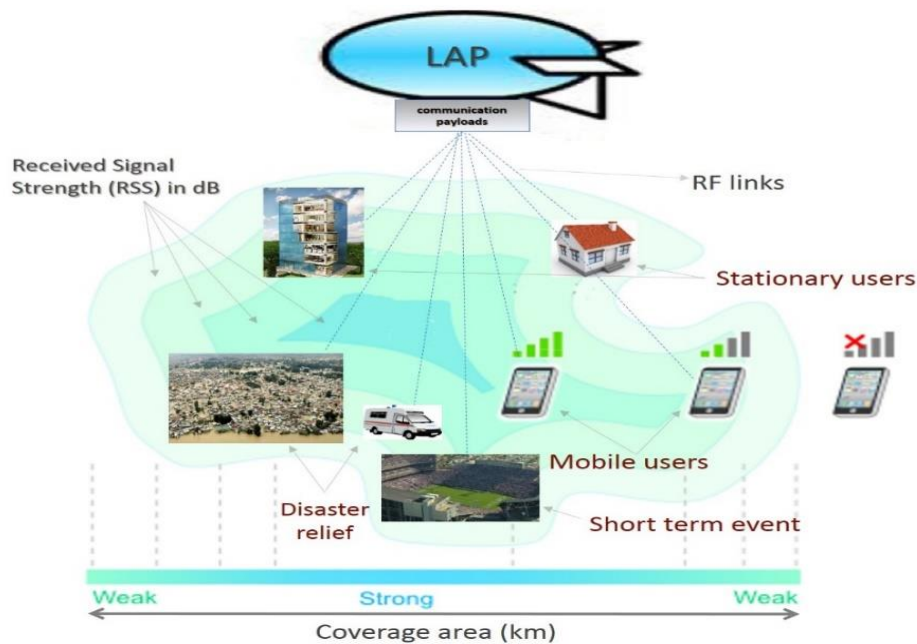
Figure 1.3: A standalone aerial platform topology
