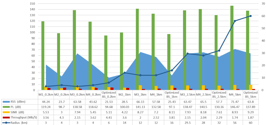
Figure 4.21: Optimised parameters in comparison to predictions with the four adapted models in a suburban environment – BS
