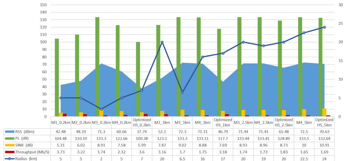
Figure 4.24: Optimised parameters in comparison to predictions with the four adapted models in a rural environment – HS
