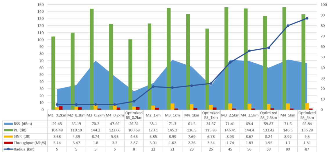
Figure 4.23: Optimised parameters in comparison to predictions with the four adapted models in a rural environment – BS
