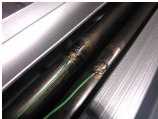
Figure 3.34 – Brazed thermocouple on thermosyphon outer wall.
