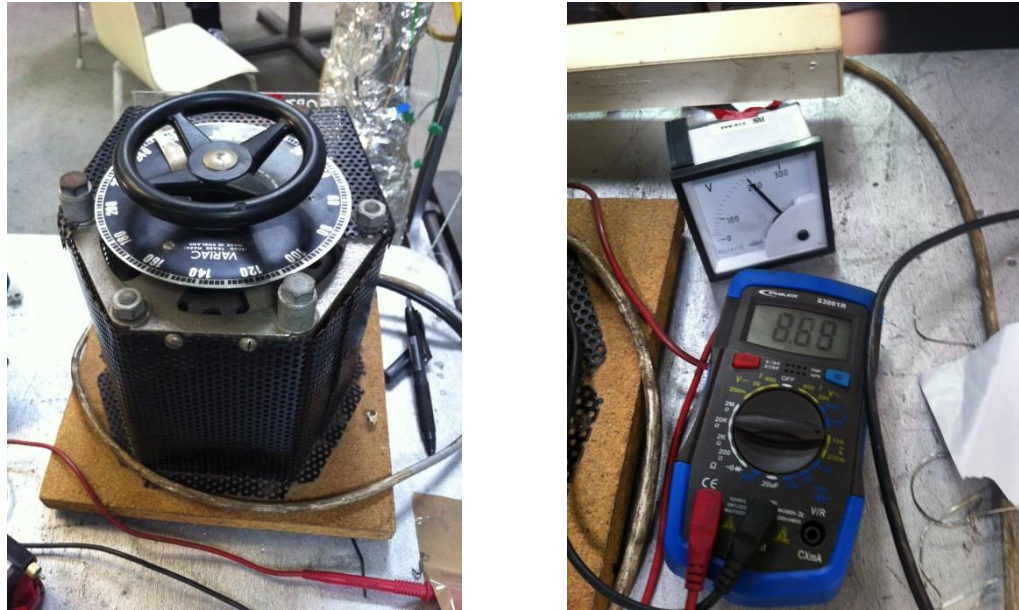
Figure 3.27 – variac (left), ammeter and voltmeter (right).
