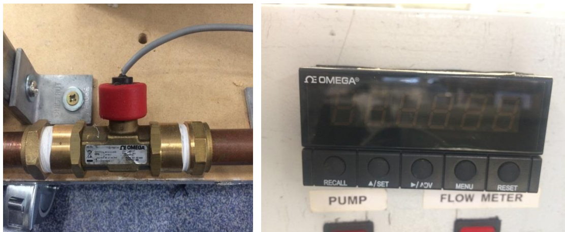
Figure 3.28 – Turbine flow sensor (left), ratemeter (right).
