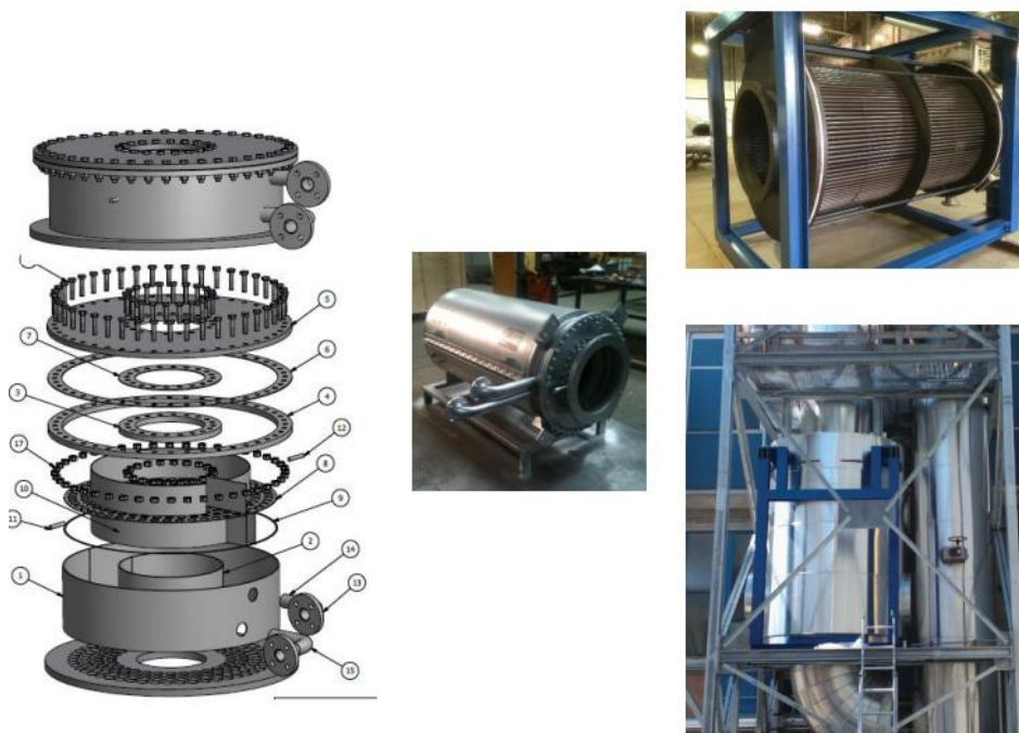
Figure 1.2 – The through flow unit designed by Jouhara [9,10].
