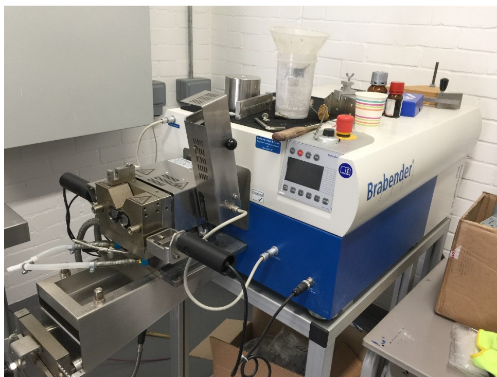
Figure 3.2 Brabender Plastograph twin-screw mixer
