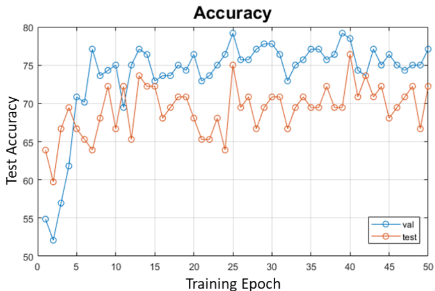
Figure 4.10 - Example of the Training process for the Medium size Deep Network on the Mouth. The Validation and Test accuracies are plotted throughout the 50 epochs of training.
