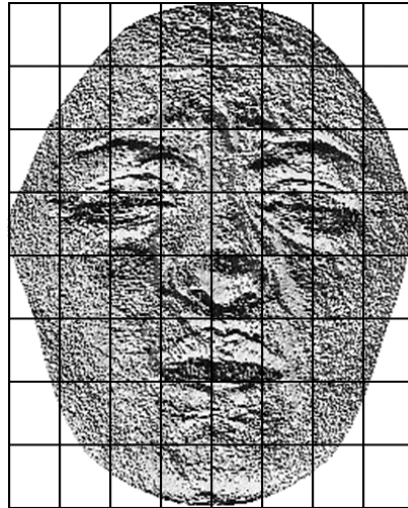
Figure 3.2 - Visualisation of the ULBP operator applied to a Facial image demonstrating an intense Angry expression, where a histogram will be produced on each of the 64 windows to make the ULBP feature
