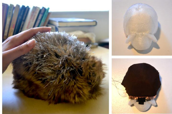
Figure 5.8 - An affective touch-sensing zoomorphic prototype with pressure and conductive sensors attached to the device, inner Styrofoam and skeleton [157].
