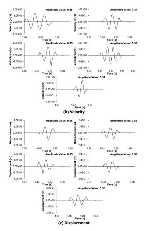
**Figure 8.4** (continued) Transient vibrations of Tarmac surface identified and extracted within the target frequency interval of 20 to 60 Hz for the first (b) and double time-domain integration (c) of steering wheel acceleration vibration
