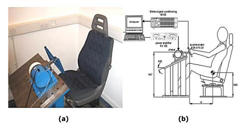
Figure 5.6 Facility used for laboratory tests, available at Human Centred Design Lab, Brunel University
