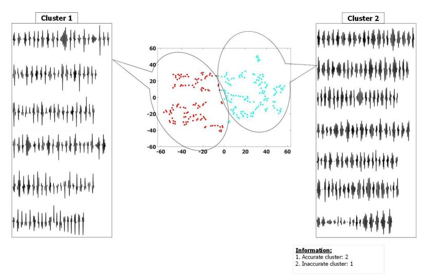
Figure 9.7 Classification of transient vibrations of 7 vibrational statistics of time-domain features
