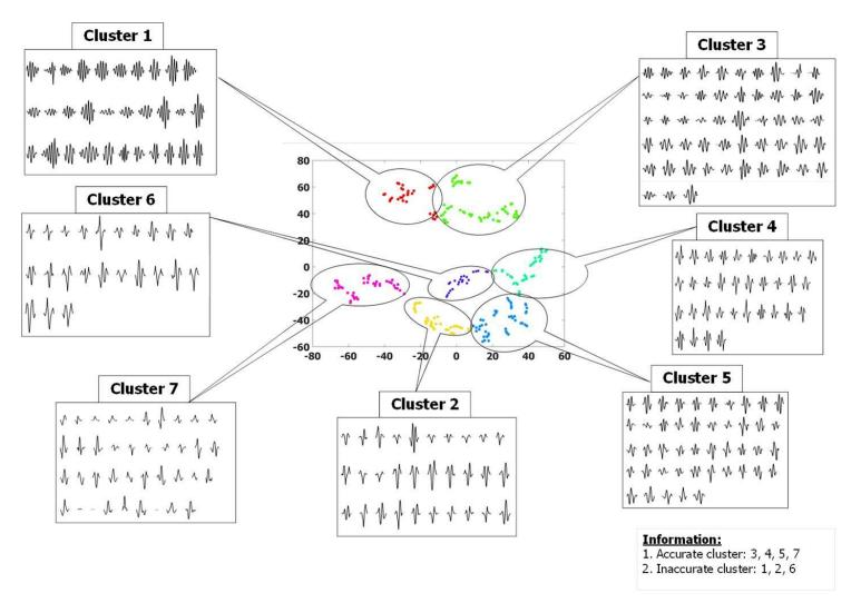
Figure 9.8 Classification of transient vibrations of 89 original time-domain features (1Δt, 88amplitudes)
