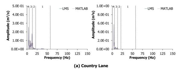
Figure 8.3 Comparison PSD showing the four wavelet groups distribution between first (left) and double time-domain integration (right) of steering wheel acceleration by LMS® CADA-X 3.5E software and MATLAB R2014a software
