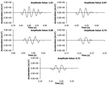
(b) Acceleration by double differentiation of displacement
