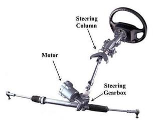
Figure 1.3 Electric power steering system (Source: Harter et al., 2000)
