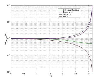
Figure 8.1 The comparison of the magnitudes of the accuracy transfer function (Source: Worden, 1990; Smyth and Pei, 2000)
