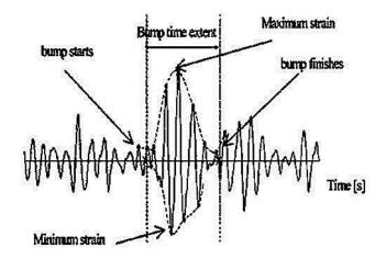
Figure 6.2 Decay envelope of the transient vibrations (Source: Giacomin and Berber-Solano, 2006)
