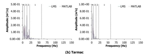
**Figure 8.3** (continued) Comparison PSD showing the four wavelet groups distribution between first (left) and double time-domain integration (right) of steering wheel acceleration by LMS® CADA-X 3.5E software and MATLAB R2014a software
