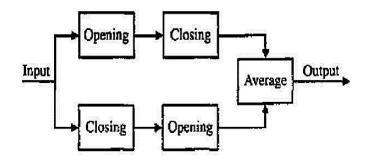
Figure 6.5 Diagram of morphological filter (Raphisak et al., 2004)
