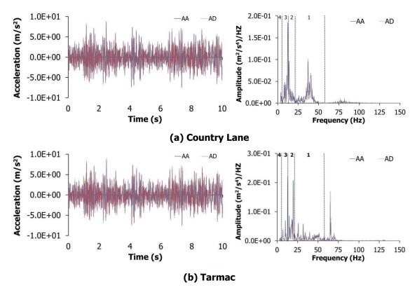
**Figure 8.6** Comparison of time histories and PSD between original acceleration by accelerometer and acceleration by double time-domain differentiation of displacement
