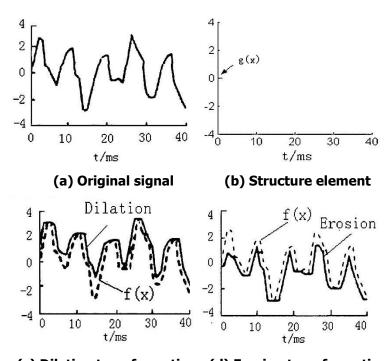
(c) Dilation transformation (d) Erosion transformation Figure 6.4 Morphological approach to signals using a flat structuring element (Source: Jing *et al.*, 2006)
