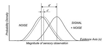
**Figure 3.4** Theoretical probability distributions of 'noise' and 'signal plus noise' for two different values of signal strength (Source: Baird and Noma, 1978)
