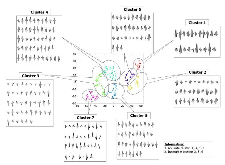
Figure 9.10 Classification of transient vibrations of 91 time-domain features (1 $\Delta$ t, 88amplitudes, 1*r.m.s*, 1Kurtosis).
