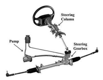
Figure 1.2 Hydraulic power steering system (Source: Harter et al., 2000)
