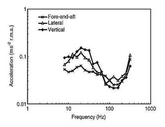
Figure 2.7 Median perception threshold contours overlaid between the three axes (Source: Morioka and Griffin, 2006)
