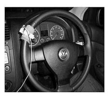
Figure 5.1 Position of steering wheel measurement point (Source: Berber-Solano, 2008)
