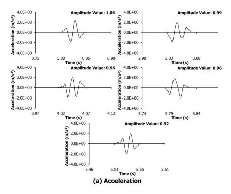
Figure 8.4 Transient vibrations of Tarmac surface identified and extracted within the target frequency interval of 20 to 60 Hz for original steering wheel acceleration vibration
