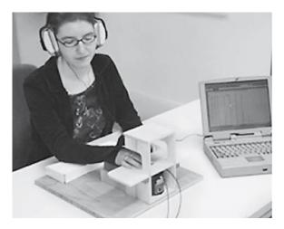
Figure 3.10 Presentation of vibrations through the vibrator embedded in a small frame house (Source: Pongrac, 2008)
