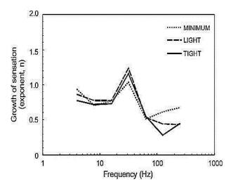
Figure 2.9 Effect of frequency and grip force on median of growth of sensation (Source: Morioka and Griffin, 2007)
