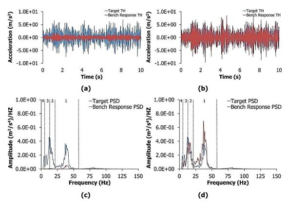
Figure 5.7 Comparison between target and bench response of time history and PSD before (a & c) and after (b & d) the compensation process.
