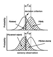
Figure 3.5 The signal detection diagram (Source: Heeger, 1998)
