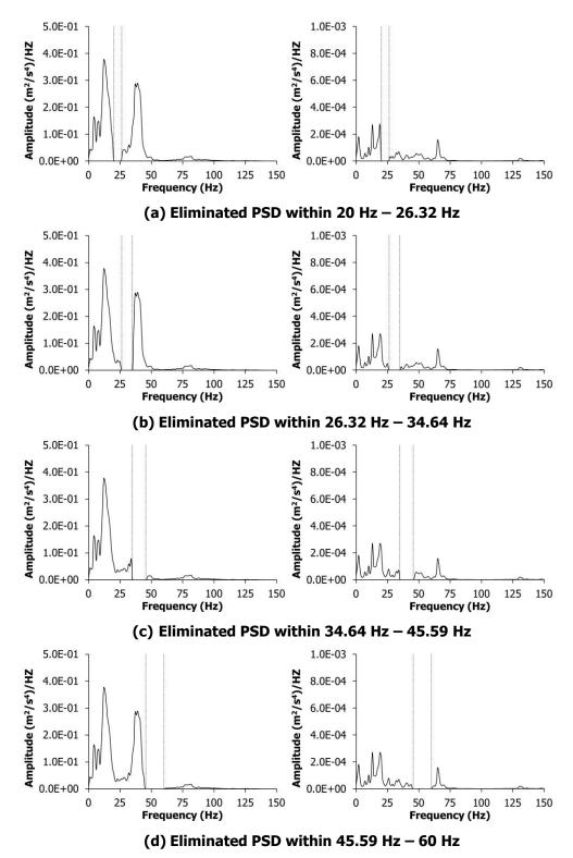
Figure 7.1 Example of original and manipulated Butterworth filter of Country Lane (left) and Tarmac (right) road surfaces used in the laboratory test stimuli
