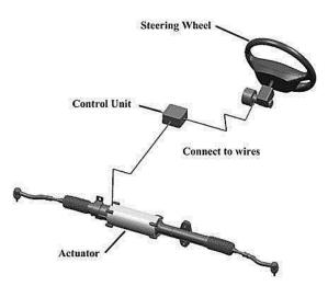
Figure 1.4 Steering-by-wire power system (Source: Berber-Solano, 2008)
