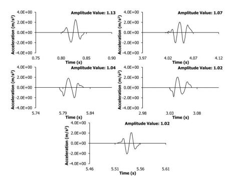
Figure 8.7 Transient vibrations of Tarmac surface identified and extracted within the target frequency interval of 20 to 60 Hz for the acceleration by double time-domain differentiation of displacement
