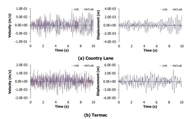
**Figure 8.2** Comparison time histories between first (left) and double (right) timedomain integration of steering wheel acceleration by LMS® CADA-X 3.5E software and MATLAB R2014a software
