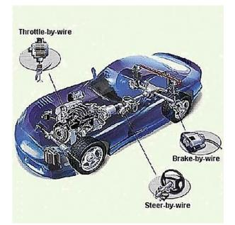
Figure 1.1 Automotive application of drive-by-wire systems (Source: KAIST, 2014)
