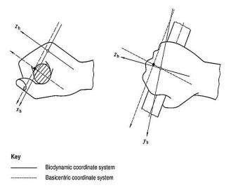
**Figure 2.6** The anatomical coordinate system for the handgrip position (Source: BS 6842, 1987; ISO 5349-1, 2001)
