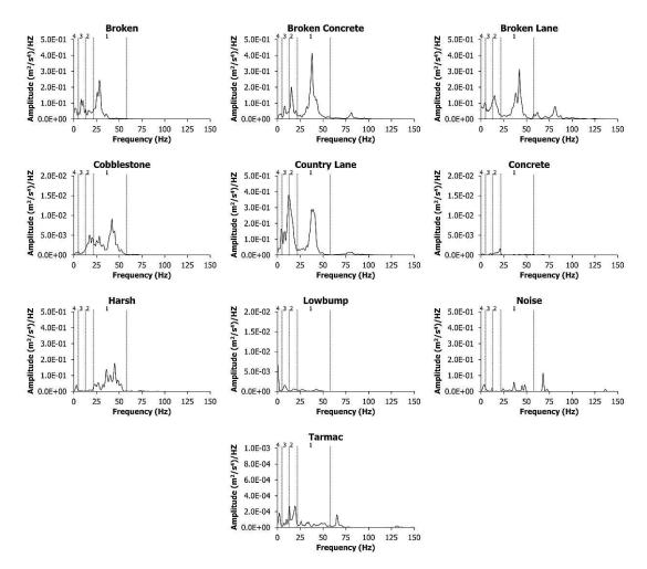
Figure 5.4 The vibration frequency-domain analysis of road surfaces by PSD
