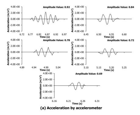
Figure 8.8 Transient vibrations of Broken surface identified and extracted within the target frequency interval of 20 to 60 Hz for the acceleration by double time-domain differentiation of steering wheel displacement vibration
