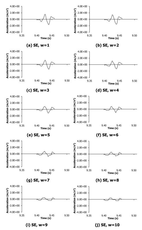
Figure 6.6 Post-processed transient vibrations results using flat structuring elements with different widths
