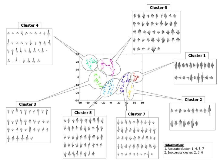
Figure 9.9 Classification of transient vibrations of 90 time-domain features (1Δt, 88amplitudes, 1r.m.s)
