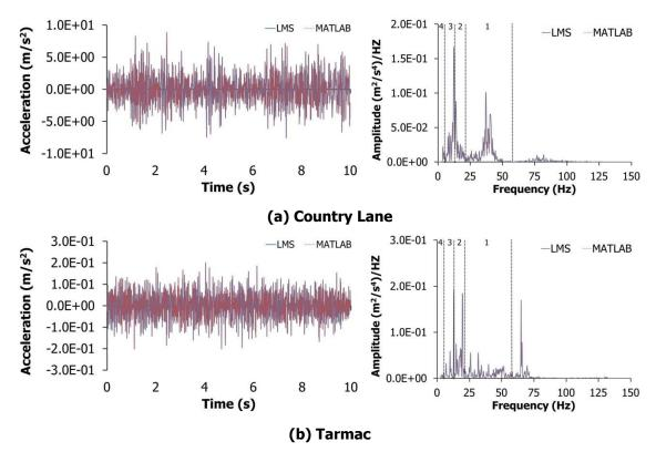
**Figure 8.5** Comparison of time histories and PSD of acceleration by double timedomain differentiation of displacement process by LMS® CADA-X 3.5E software and MATLAB R2014a software
