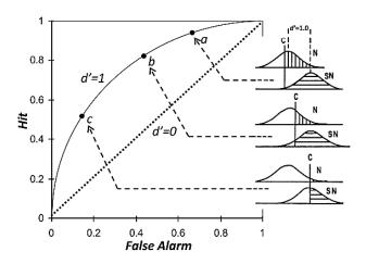
**Figure 3.8** ROC curve for the signal plus noise and the noise distribution (d'=1), obtained over different observers' criteria (Source: Green and Swets, 1966)
