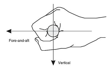
Figure 3.12 Hand posture and axis of vibration. The lateral axis is defined as parallel to the handle axis (Source: Morioka and Griffin, 2006)
