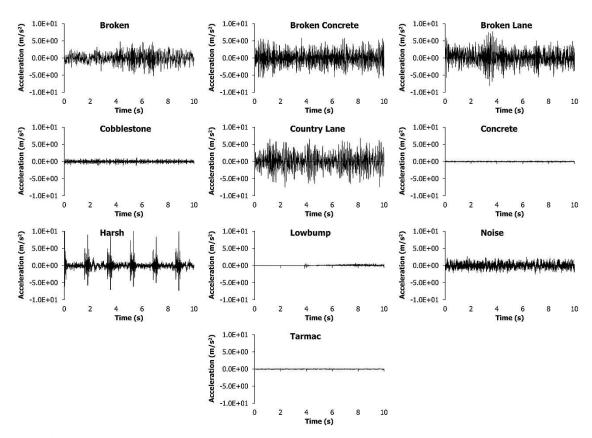
Figure 5.3 The time history segments extracted from the road test recordings for laboratory tests
