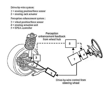
Figure 1.5 An approach of a perception enhancement system using by-wire steering (Source: Giacomin, 2005)
